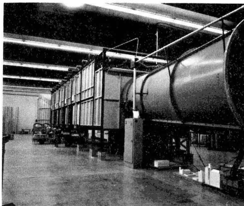
Figure 3. Exterior of Environmental Wind Tunnel.
