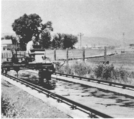
Rating tank with recording instrumentation
