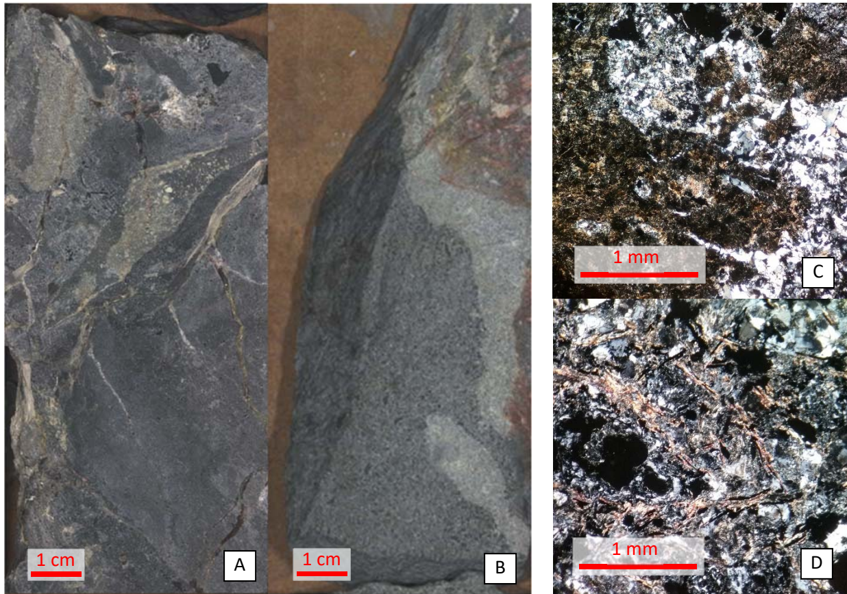
Figure 10. BD14-04C_701.2 (left and upper right) and BD14-04C_706 (center and bottom right) are samples of the Russet diorite dike. Figure A is an example of small clasts (peperite?) of diorite in the upper contact of the silicified zone and unsilicified zone of the Rodeo Creek Formation. The contacts are both igneous and faulted. Figure C is the photomicrograph from that sample. Figure B is the upper contact (intrusive) of the Russet dike into the Rodeo Creek mudstone showing the chilled margin of the dike and the baked contact of the mudstone. Figure D is the photomicrograph from that sample.
