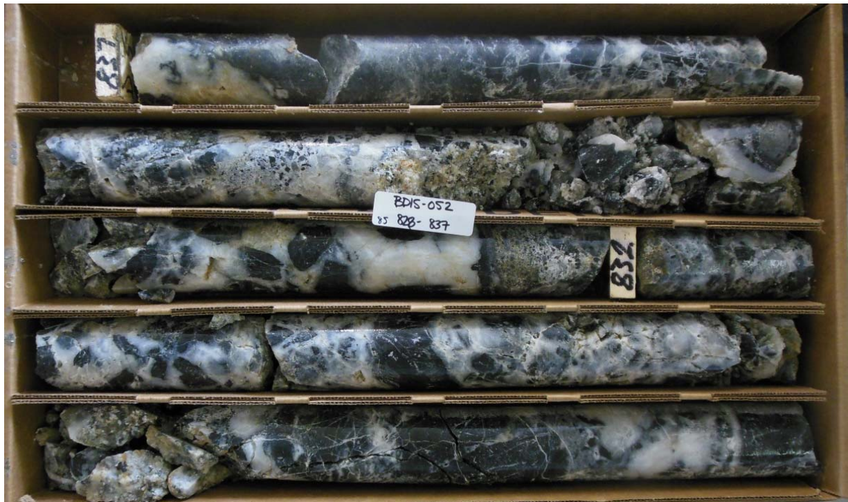
Figure 109. BD15-052, 828-837 ft. depth. Image of Bx1a, intensely silicified (clast and matrix) mudstone hydrothermal breccia which rebrecciated Bx1
