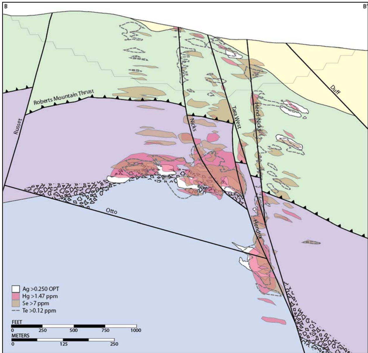
Figure 70. Cross-section through the El Niño mine with contours of silver enrichment (>0.250 opt) compared to mercury (>1.47 ppm), selenium (>7 ppm), and tellurium (>0.12 ppm) relative to the major faults, four major formations, breccias, and silicification zones. See Figure 7 for unit legend and drill-hole locations.
