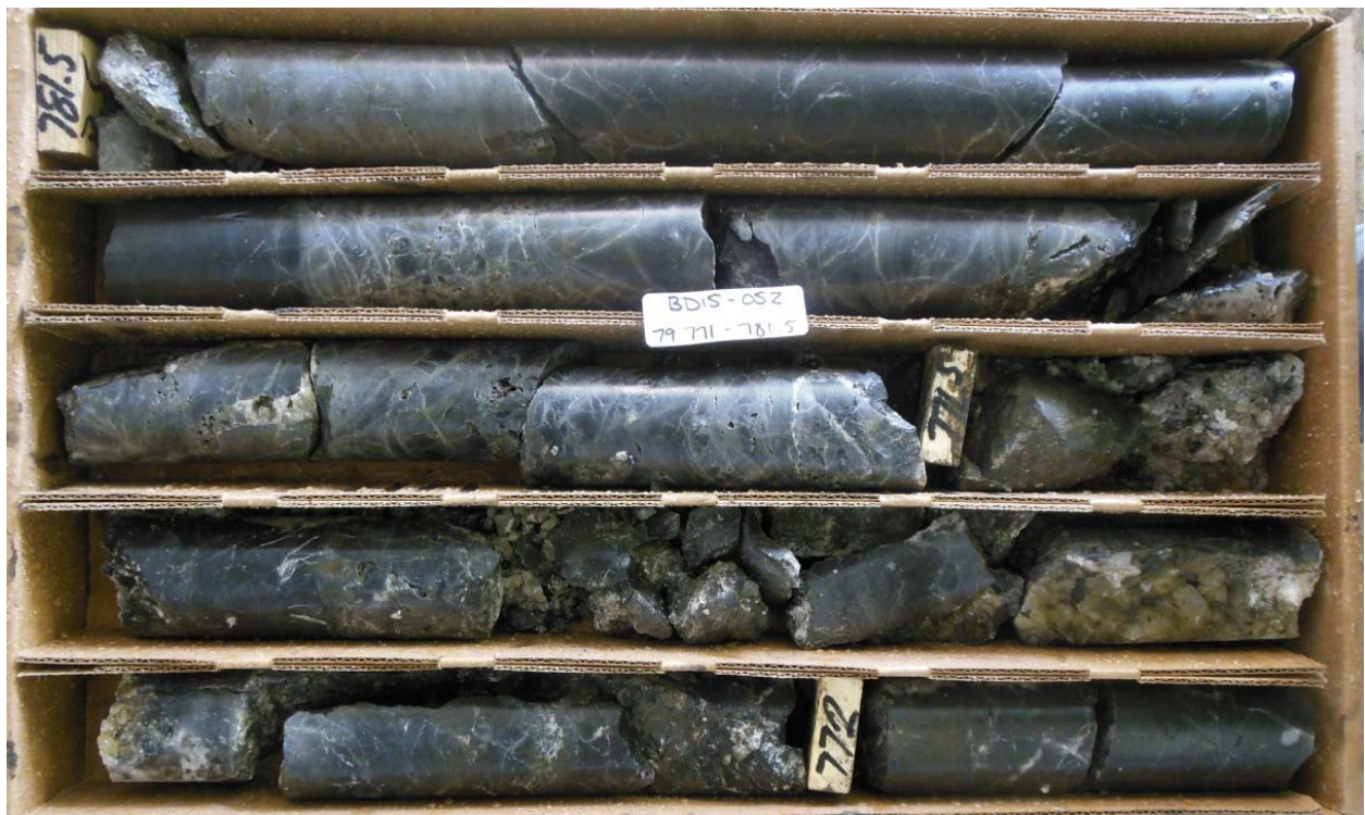
Figure 107. Drill hole BD15-052, 771-781.5 ft. depth. Image of quartz-(ammonium) sericite-pyrite altered mudstone crackle breccia (Bx3a).
