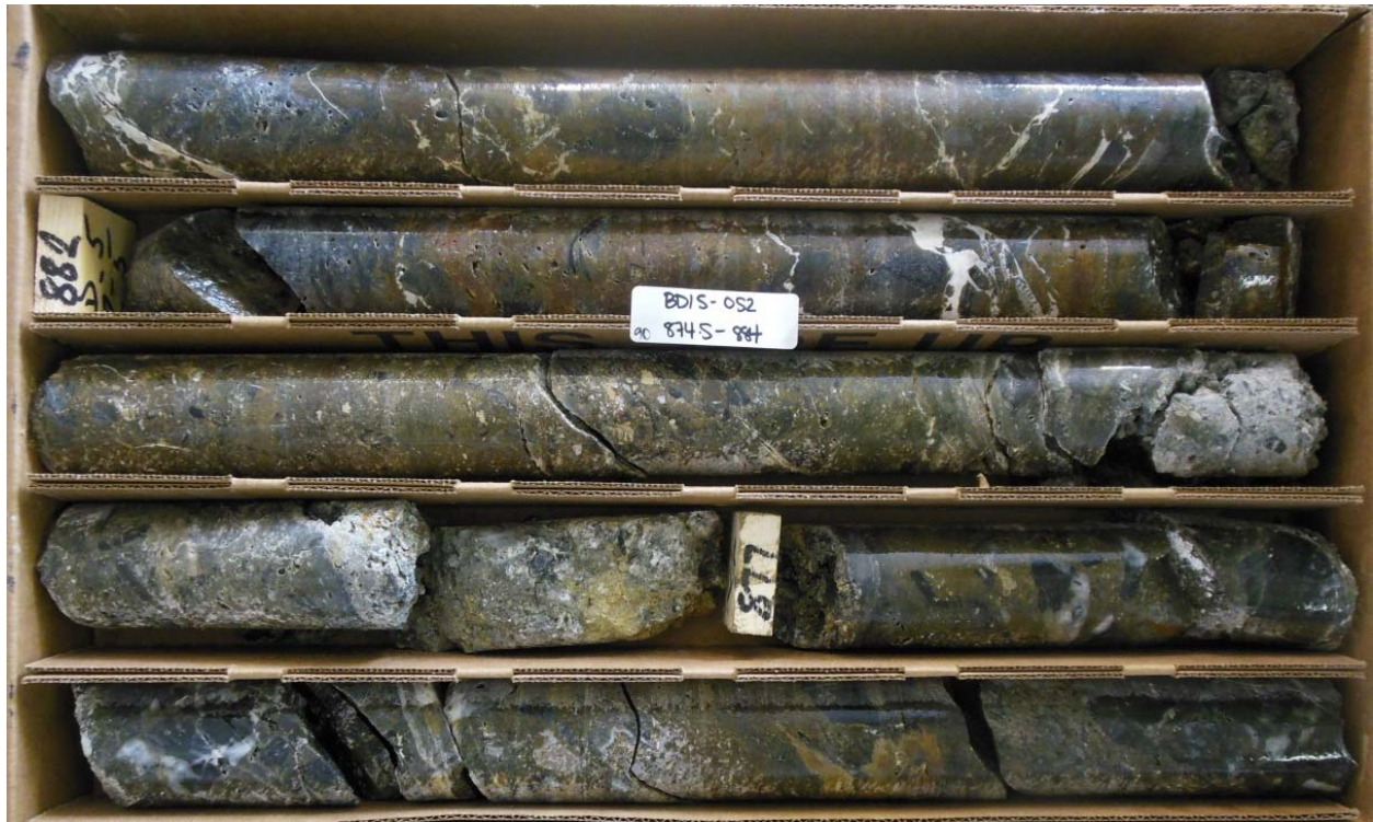
Figure 112. BD15-052, 874.5-884 ft. depth. Bx5b, decalcified, silicified, chaotic limestone clasts, matrix supported, calcite cemented collapse breccia.
