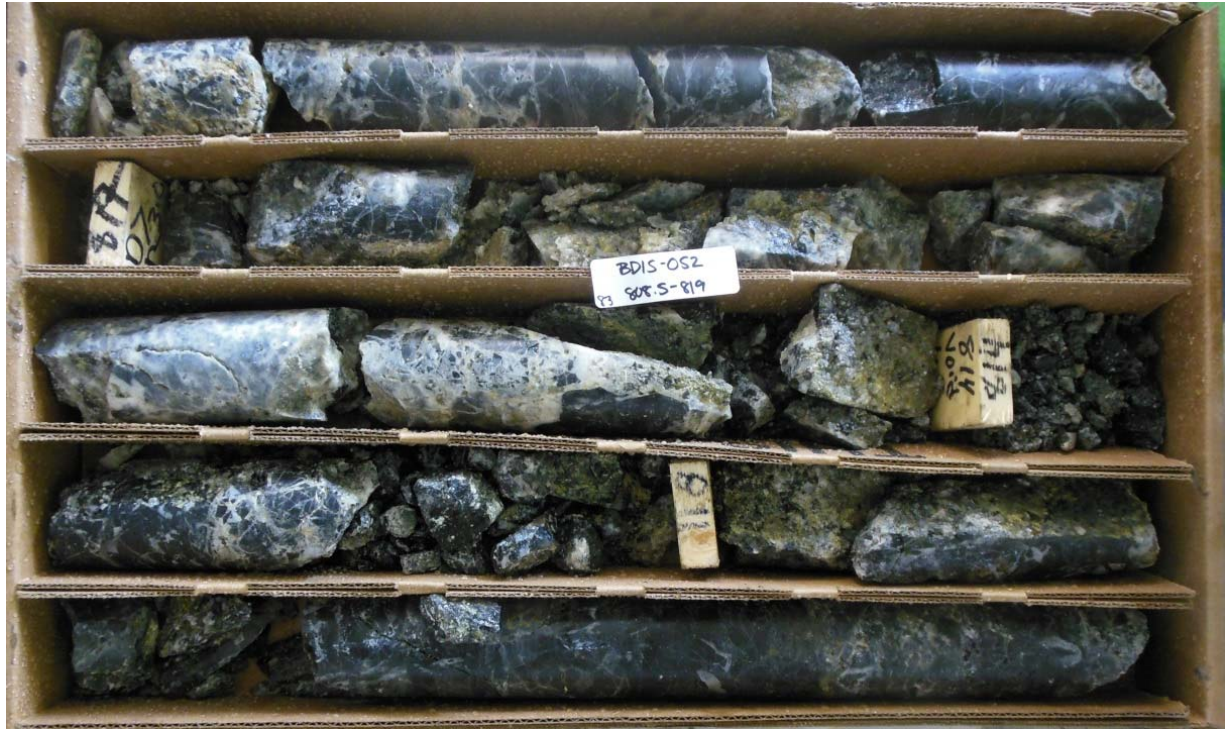
Figure 108. Drill hole BD15-052, 808.5-819 ft. depth. Image of Bx1a, intensely silicified (clast and matrix) mudstone/limestone hydrothermal breccia which rebrecciated Bx1 and Bx2 vuggy silica cemented hydrothermal breccia that rebrecciated Bx1 tectonic breccia.
