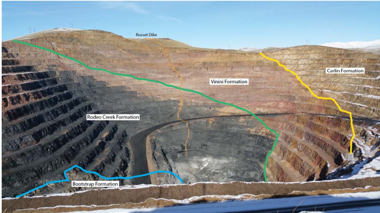
Figure 8. Arturo pit looking north-northwest. The blue line represents the top of the exposed Bootstrap Formation, green is the approximate top of the Rodeo Creek Formation, yellow is the top of the Vinini Formation, above which is the Carlin Formation. The orange line shows where the Russet Dike outcrops in the Arturo pit.
