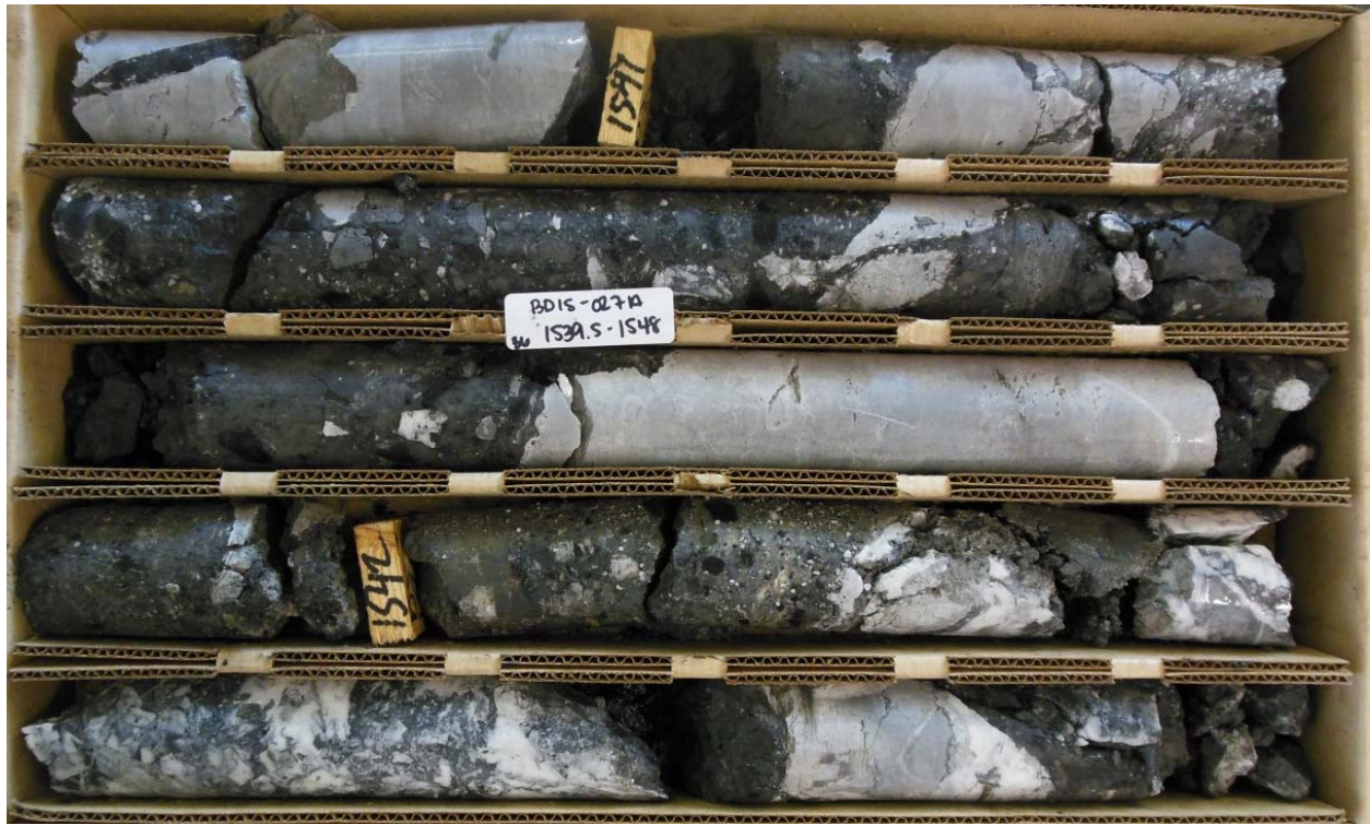
Figure 111. BD15-027A, 1539.5-1548 ft. depth. Image of Bx5a unsilicified dissolution collapse breccia.
