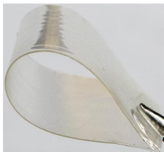
Figure 3.11. Photograph of solvent casted and photocured st -PVMA- hν film (0.06 mm thick).
