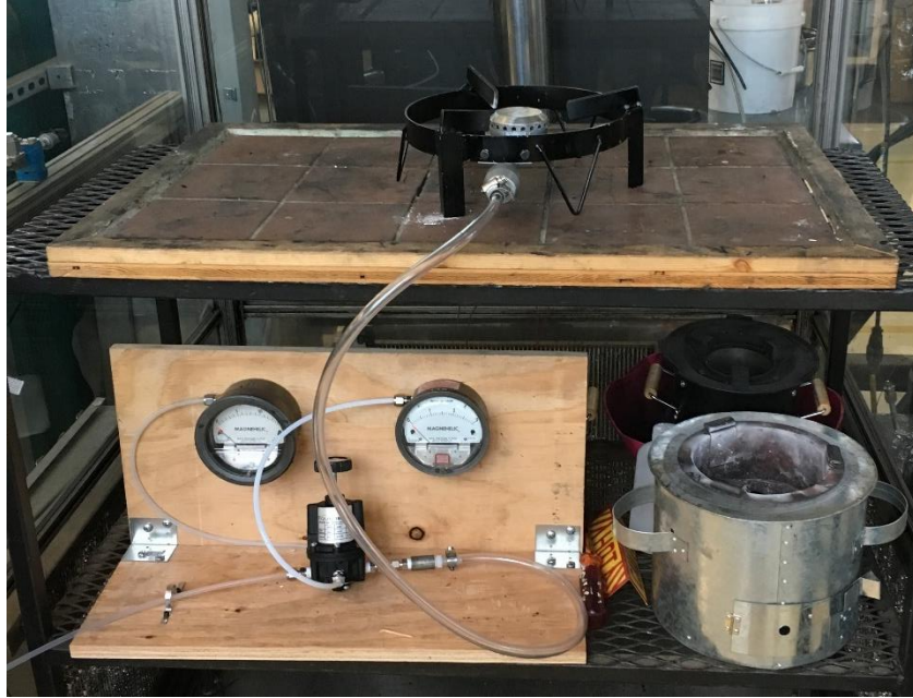
Figure 15 – Combined with a cylinder scale, the regulator provides flow control adjustment while the Magnehelic gauges provide supply pressure monitoring
