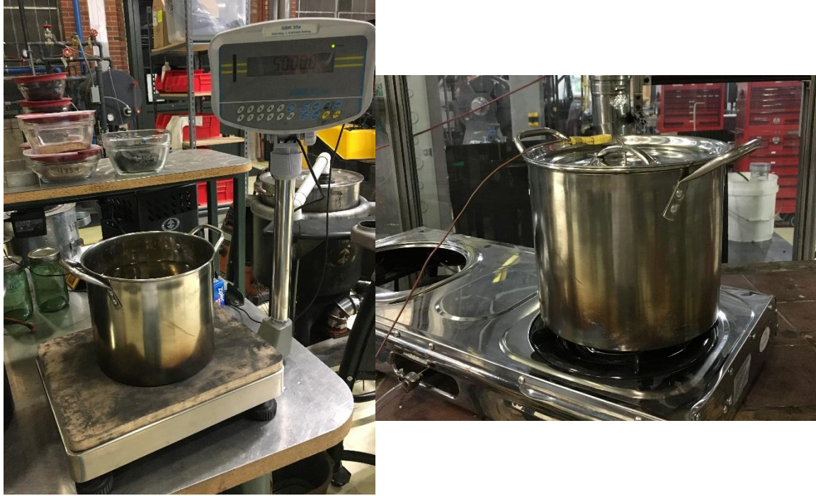
Figure 22 – Left: Measuring 5L of water, Right: Placement of an Omega K-Type thermocouple through the pot lid for the duration of each test
