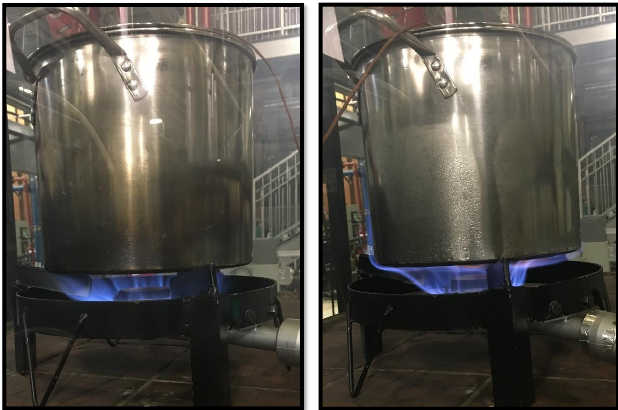
Figure 34 – Left: Partially premixed flame, Right: Diffusion flame
