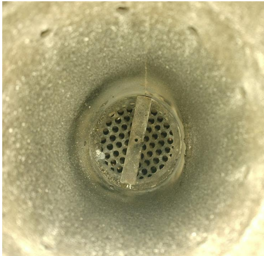
Figure 3: Ash grinder blade inside of combustor
