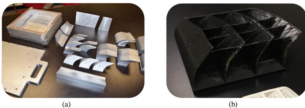
Figure 3: The tooling (a) required to create a composite cascade basket (b) is one of the barriers to widespread use of composites.
