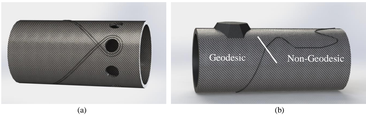
Figure 2: Non-geodesic fiber paths are shown in (a) and (b). Localized buildup of material is also shown in (b).
