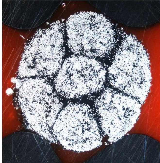
Figure 11: The cross-section of a fiber rod shows a hexagonal yarn packing with high fiber volume fraction and low void content [17].
