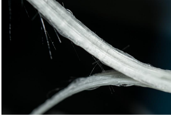
Figure 64: Fiber pullout was evident in most of the adherend surfaces after peeling occurred.
