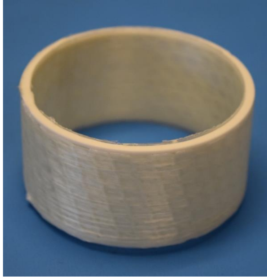
Figure 80: The de-tooled honeycomb composite with edge closeouts and a minimal amount of flash.
