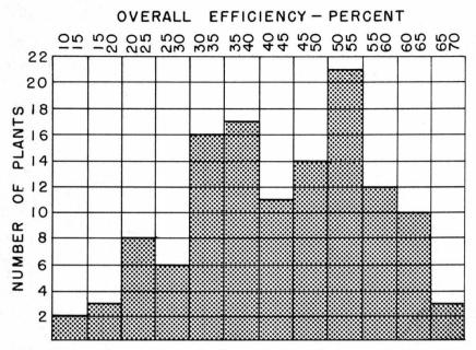
FIGURE 4.—Distribution of overall efficiency values of pumps tested.
