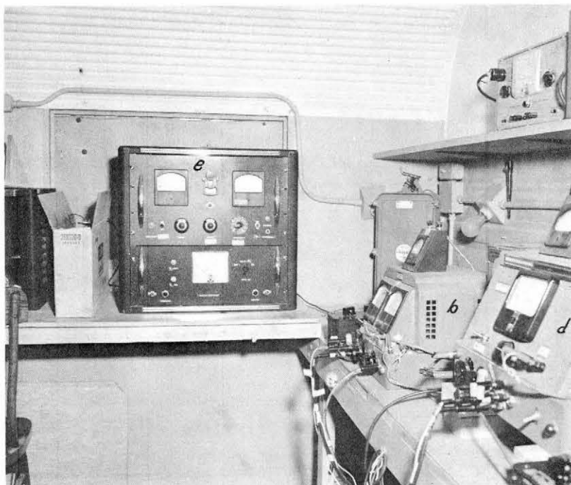
Fig. 9 Views of Instrument b Hot-wire anemometer No. 1 d Hot-wire anemometer No. 2 e Resistance thermometer
