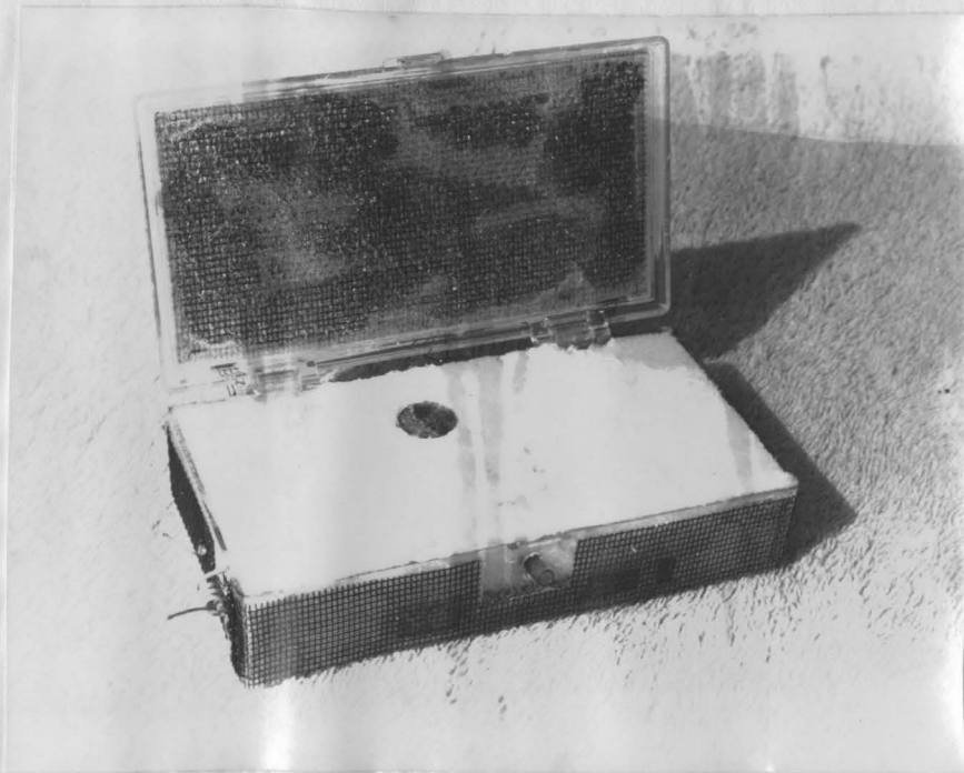
Fig. 7 Capacitance probe transmitter after encapsulation. A brass heat-sink is mounted over the transistor. The battery is externally mounted being connected to the wires at the left.
