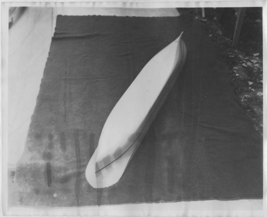
Fig. 5 View of the bottom of the model, showing the location of the pressure gages.
