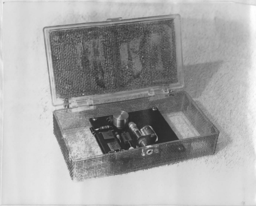
Fig. 6 Capacitance probe transmitter unit before encapsulation. The two-inch square plate is located under the transmitter. Tuning is accomplished by turning the adjustment screw of the small piston capacitor through the hole in the front of the case.
