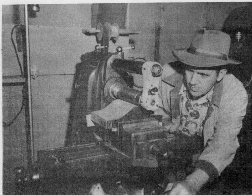
Fig. 4.10 Photograph of milling of bottom contour of model hull
