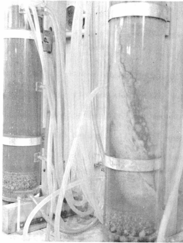
Fig. 4 Bentonite suspension by-passes the soil column at boundary (Series V Run B).
