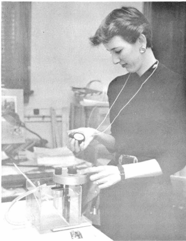
Fig. 30 Viscosity determination of bentonite suspension.
