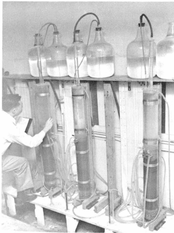
Fig. 3 Collection of data during run (Series VI). Note the different sized graduated cylinders needed for various hydraulic gradients.
