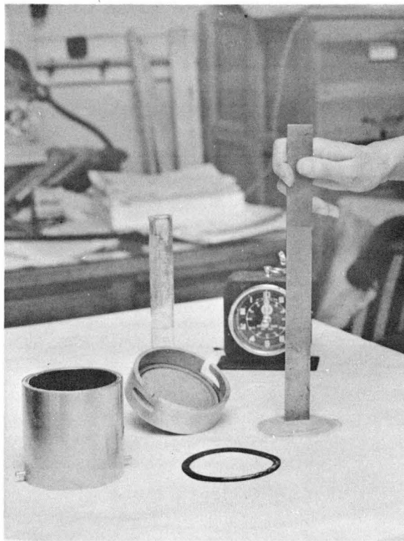
Fig. 29 Measuring the filter cake thickness in the wall-building evaluation of bentonite.
