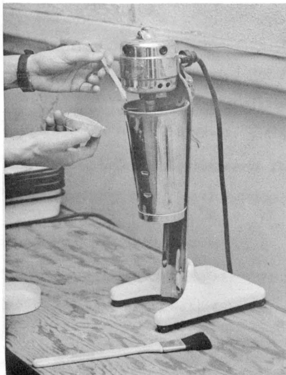
Fig. 27 Preparation of a 6-per cent bentonite suspension by the use of a high-speed rotary beater.
