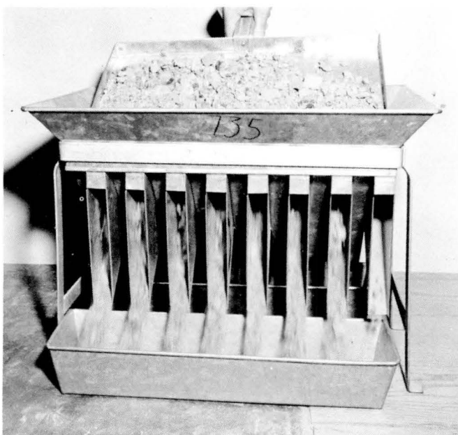
Figure 25.—Splitting sample into representative portions.
