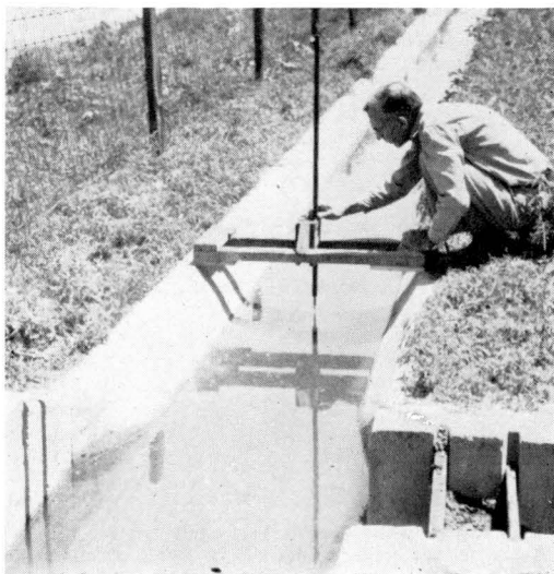
Figure 19.—Point gage being used to measure drop in water surface of pool in concrete-lined section of farm lateral, College East Farm, Fort Collins, Colorado.
