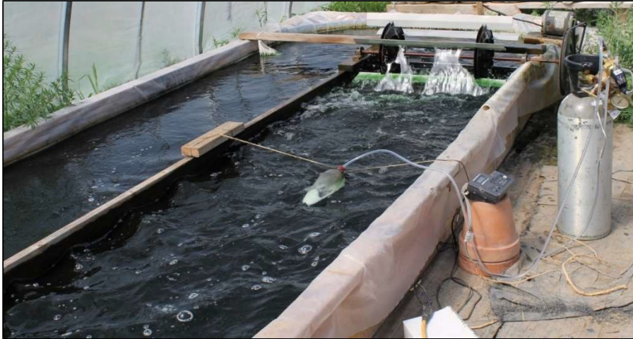
Figure 19. Raceway and CO 2 supplementation setup for on-farm high tunnel production of Anabaena sp.
