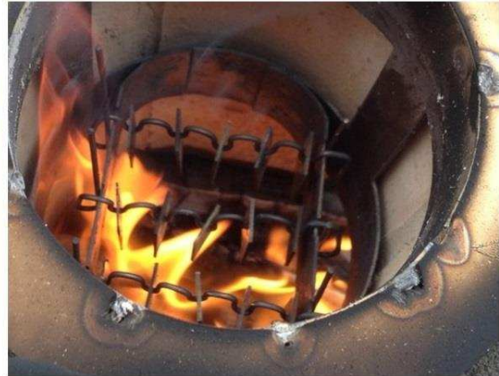
Figure 2: Photographs of coupons in (a) lab furnace test and (b) in-situ cookstove test.
