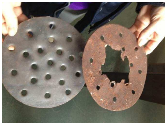
Figure 1: Charcoal stove fuel grates, new (left) and corroded (right).
