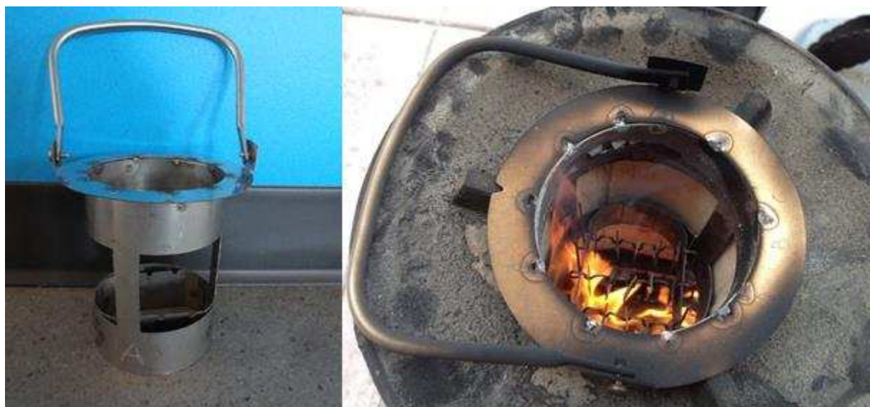
Figure 14: Fixture for hanging coupons inside stove.
