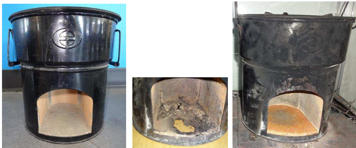
Figure 19: Stove B before testing (left), at 550 hours - before repair (middle), and after repair (right).
