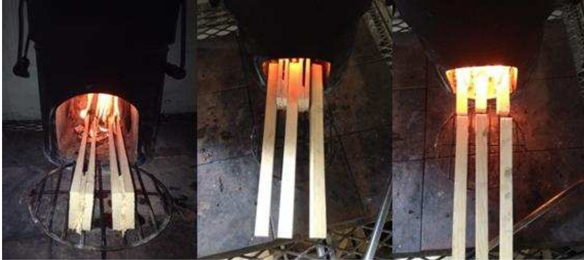
Figure 18: Startup of stove using shim packs, transition from shim packs to sticks, and transition from one set of sticks to the next.
