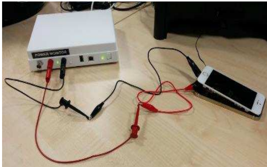
Fig. 4.6 Monsoon power monitor setup
