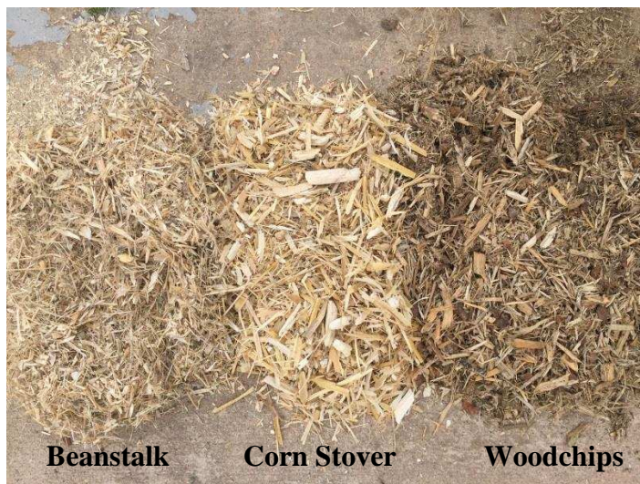
Figure 11 - Examples of Bulking Material Used
