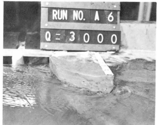
Figure 38 (c). Modification R-3. Some minor reduction in turbulence and draw-down was noticed.
