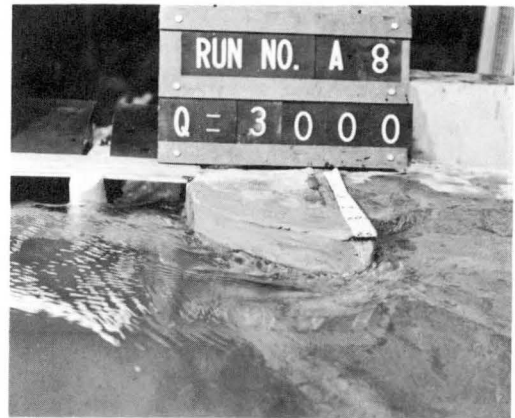
Figure 38 (b). Modification R-2. The turbulence not materially reduced. Little improvement in flow condition was noticed.
