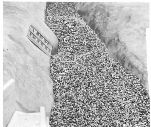
Figure 60 (b). Scour patterns with 3/4-inch gravel. Q = 2000 cms.
