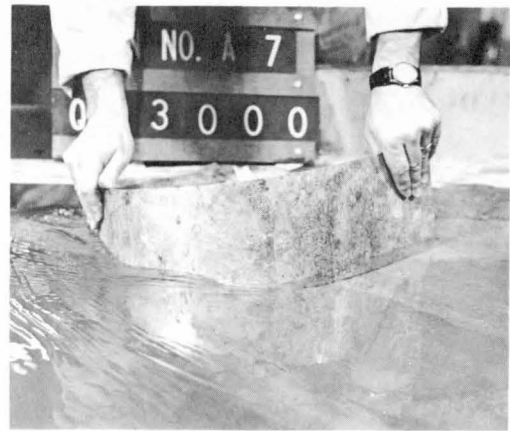
Figure 39 (b). Extension of modification R-3. Flow is smoother along the wall.
