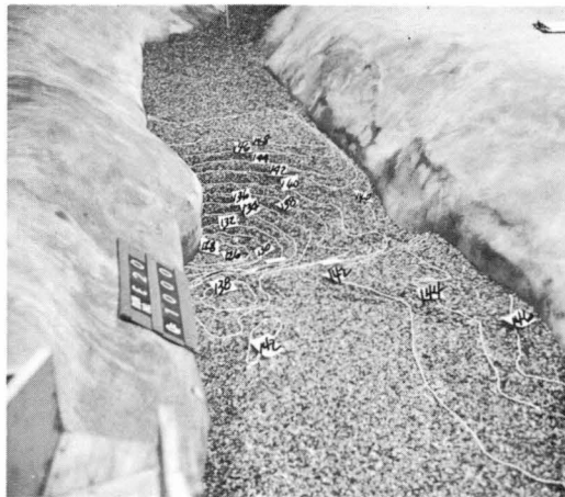
Figure 54 (a). Scour pattern with 3/8-inch gravel Spillway Q = 2000 cms Power Plant Q = 0 Model Time = 45 minutes Maximum scour depth = 126.0 m Beginning river level = 140.6 m
