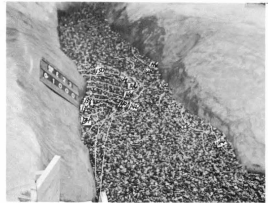
Figure 60 (a). Scour patterns with 3/4-inch gravel. Q = 1000 cms.
