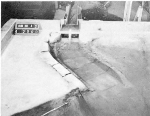
Figure 35 (b). Preliminary channel cut. Notice the rough water surface along the right bank where velocity over the cut is high and a horizontal vortex along the bank is created.
