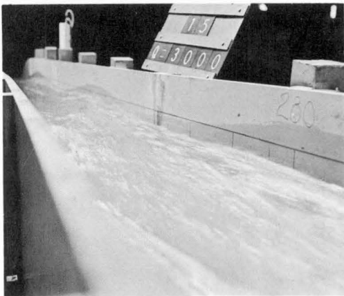
Figure 25 (c). Pier extension of 15 meters (looking downstream). Some reduction in wave height from the preliminary pier is evident.
