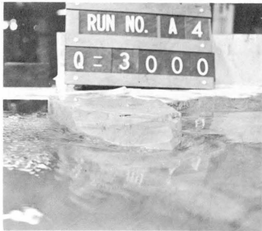
Figure 38 (d). Modification R-4. Turbulence was reduced, but draw-down at the beginning of the wing wall remained about the same as previous modifications.
