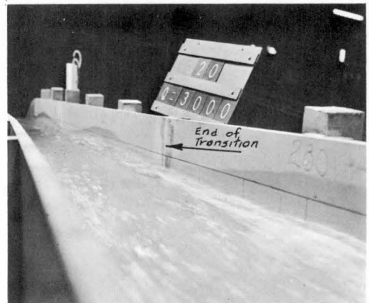
Figure 25 (d). Pier extension of 20 meters. Definite reduction in height of standing waves. The wet line seen on the wall is from previous tests.
