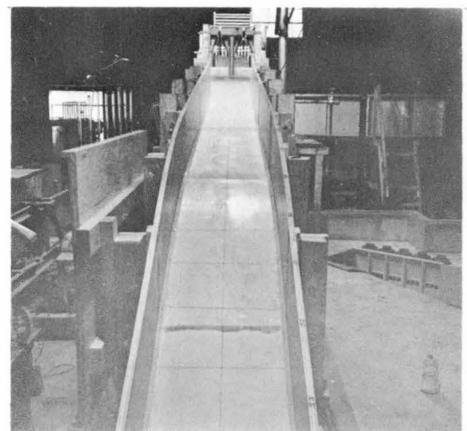
Figure 9. Completed chute model as viewed from the downstream end of the chute. The lateral lines are 10-meter markers used to aid laboratory measurements.
