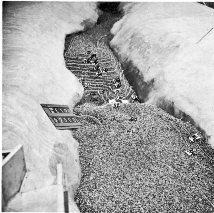
Figure 55 (a). Scour pattern with 3/8-inch gravel Spillway Q = 2000 cms Power Plant Q = 400 cms Model Time = 38 minutes Maximum scour depth = 124.0 m Beginning river level = 140.6 m
