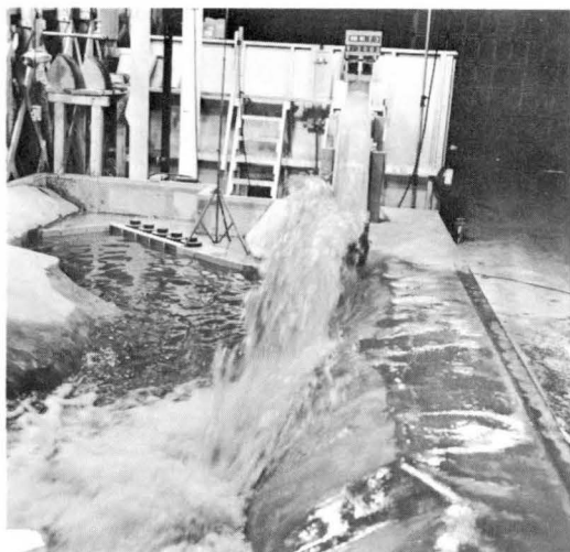
Figure 43 (b). Preliminary design. Q = 3000 cms. The jet deflection was inadequate.
