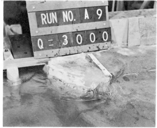
Figure 38 (a). Modification R-1 (recommended). Notice the flow over the cut bank adjacent to the wing wall.
