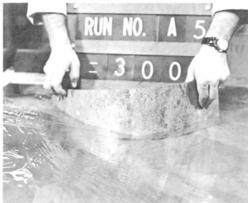
Figure 39 (a). Extension of the wing wall of modification R-4 into the reservoir. The turbulence is further diminished by a smooth transition.
