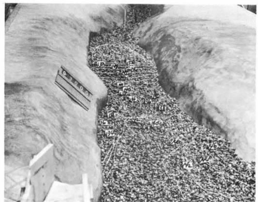
Figure 60 (c). Scour patterns with 3/4-inch gravel. Q = 3000 cms.
