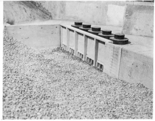
Figure 13. Completed power plant in the general model.
