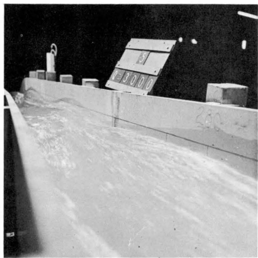
Figure 25 (a). Pier extension of 5 meters (looking downstream). Wave height remained substantially the same as that for the original pier. The painted horizontal line on the model wall indicates the top of the prototype wall.
