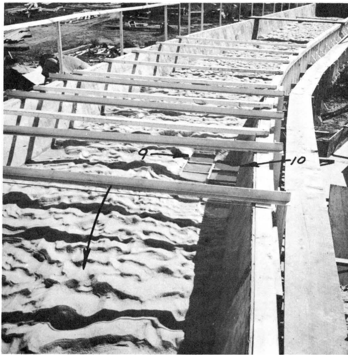
Fig. 17. Canal bed after Test Run 13 with ejectors 9 and 10 ejecting continuously. Note some scour of the downstream bins.
