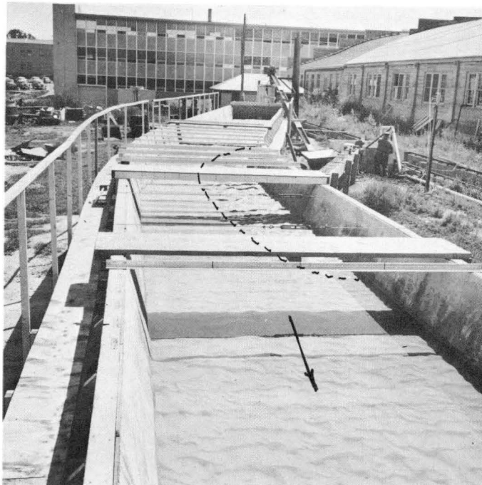
Fig. 15. Shoal formation in canal bend. Same run as Fig. 14. View is upstream.
