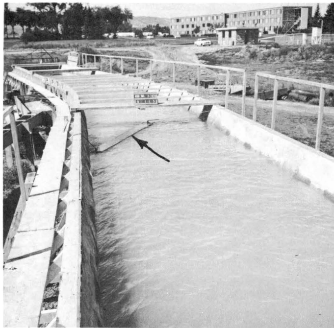
Fig. 27. Surface vane upstream of canal curve. The angle of the vane with respect to canal bank was large for this test.
