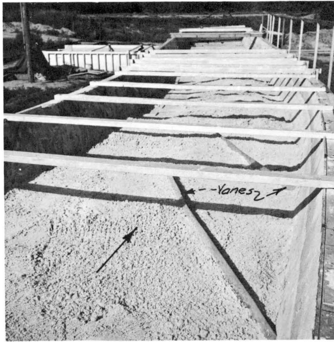
Fig. 20. Bed vanes at beginning of curve. Preparation for Run 15. Note large angle of vanes with respect to canal bank.
