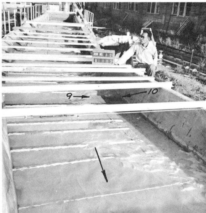
Fig. 18. Effect of grates over bins on reduction of scour. Compare with Fig. 17.
