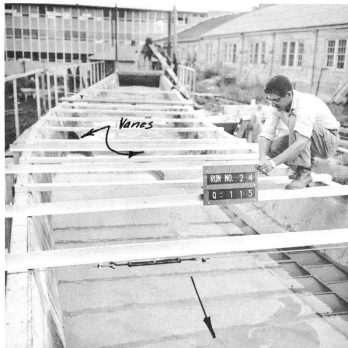
Fig. 25. Two bed vanes in the canal curve. Note scour over bins and downstream of vanes.
