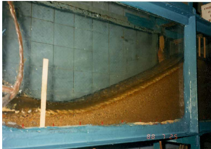
Figure 2. Test of WSBs protecting a coarse sand embankment under overtopping and seepage flow at the laboratory of MCEI (courtesy of Dr. Raymond Baker)
