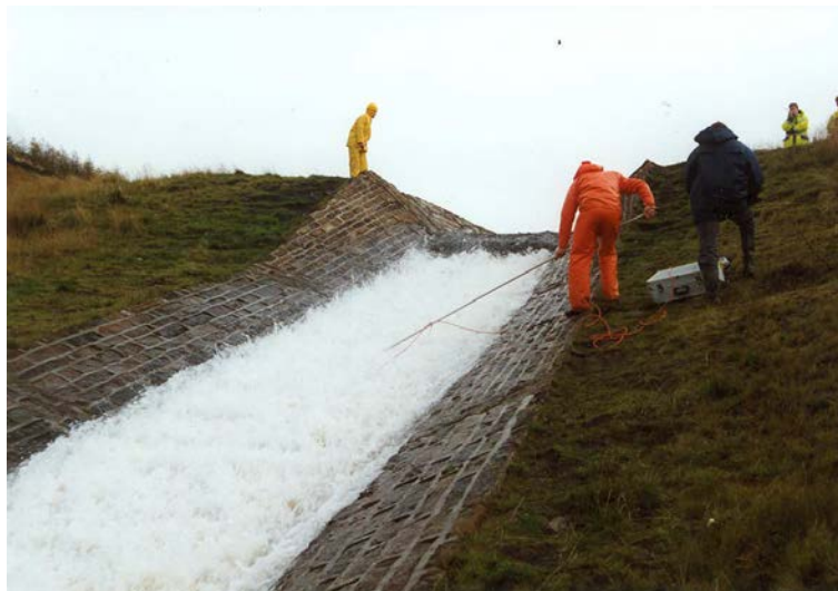
Figure 17. In site tests at Brushes Clough spillway (courtesy of R. Baker)
