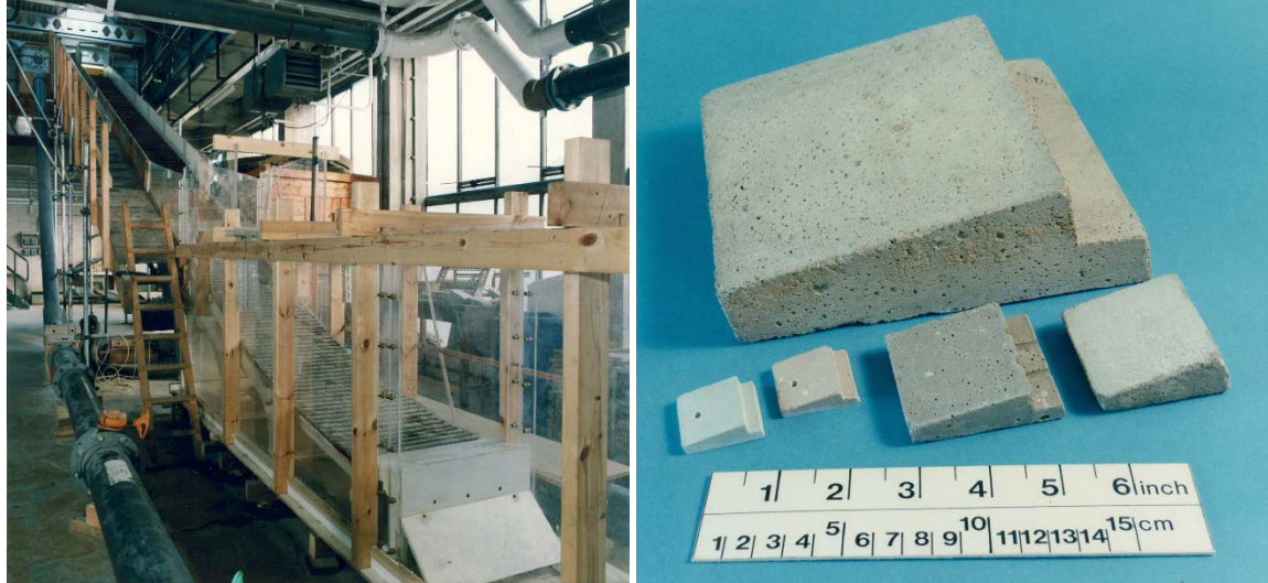
Figure 6. Experimental set up (left) and sizes of the WSBs (right) tested in Salford University (Baker 1992)
