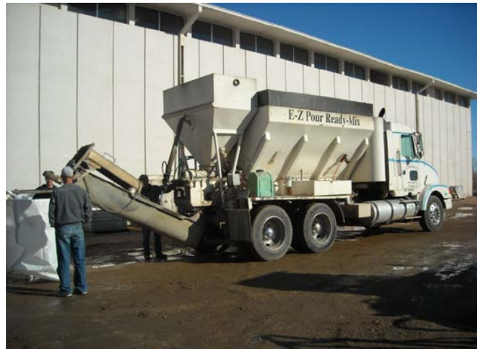
Photograph 2. Volumetric Cement Mixer (Ready-Mix Truck)
