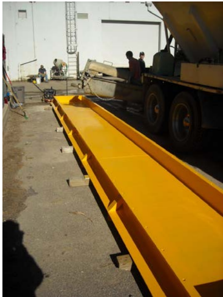
Photograph 1. Soil-Cement Test Box
