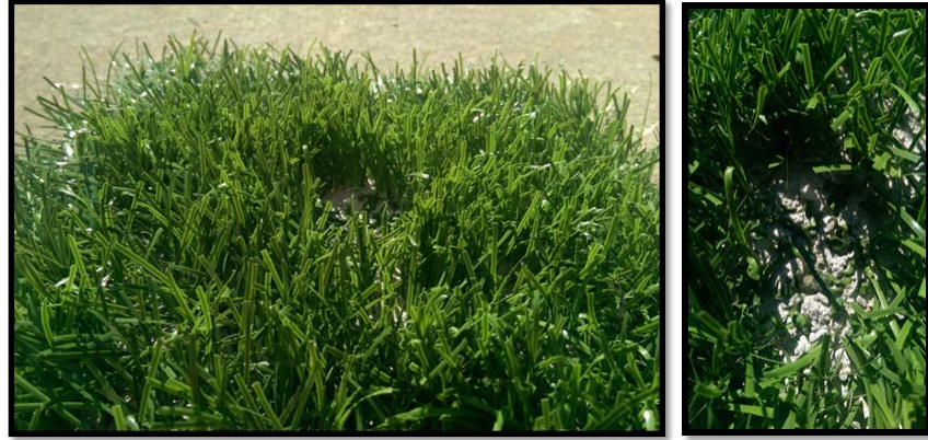
Figure 17. TGRS Sample after Flammability Testing
