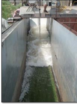
Figure 5. Hydraulic Jump Testing of TGRS
