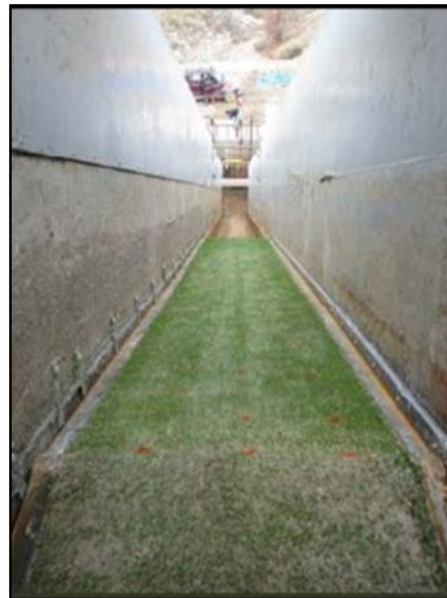
Figure 3. 5-ft Overtop Steady State Testing of TGRS
