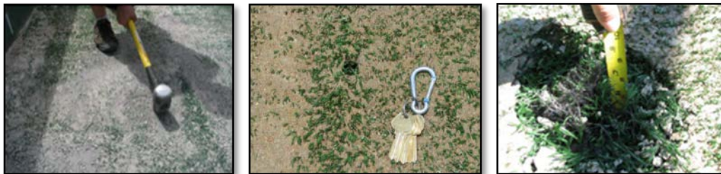
Figure 11. Intentional Damage to the TGRS: Pulverization, Simulated Bullet Hole, and Large Hole
