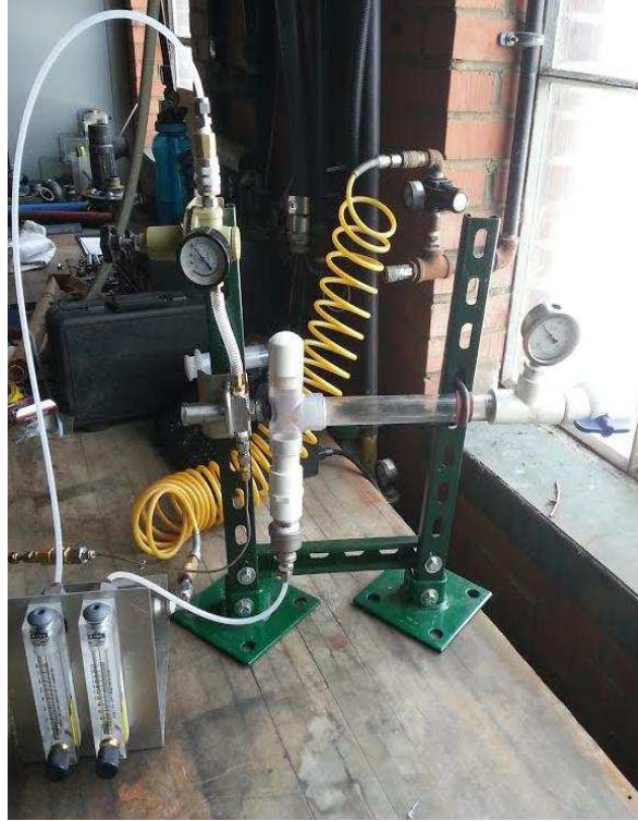
Figure 23: Low flow atomizing nozzle bench test set-up.
