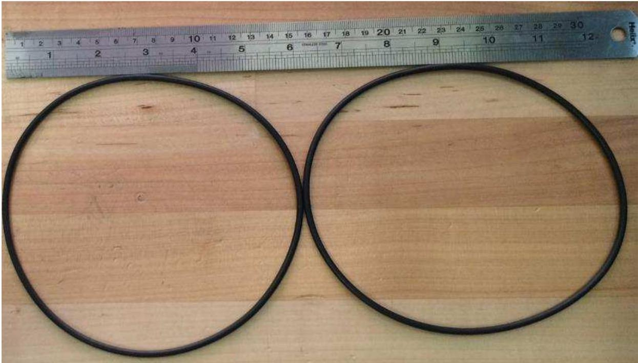
**Figure 9.7 Forward Hydraulic Oil Chamber Seals.**
