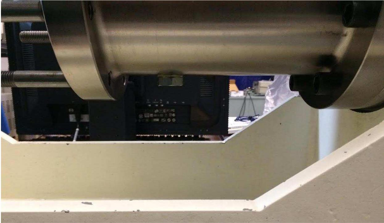
**Figure 8.7 RCM Oil Chamber Drain Plug.**
