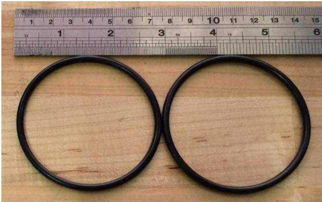
**Figure 9.15 Linear Transducer Seals.**
