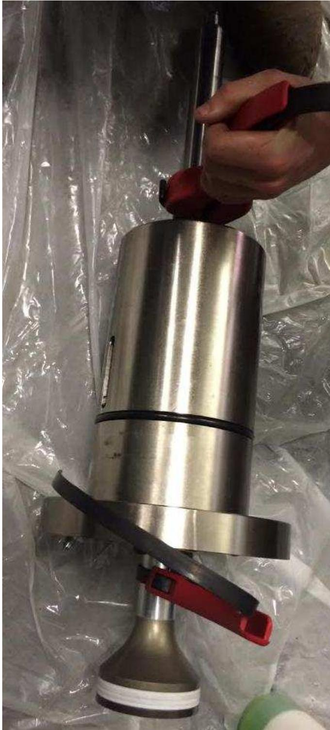
**Figure 8.12 Using strap wrenches to unscrew Compression Plunger from Drive Plunger.**
