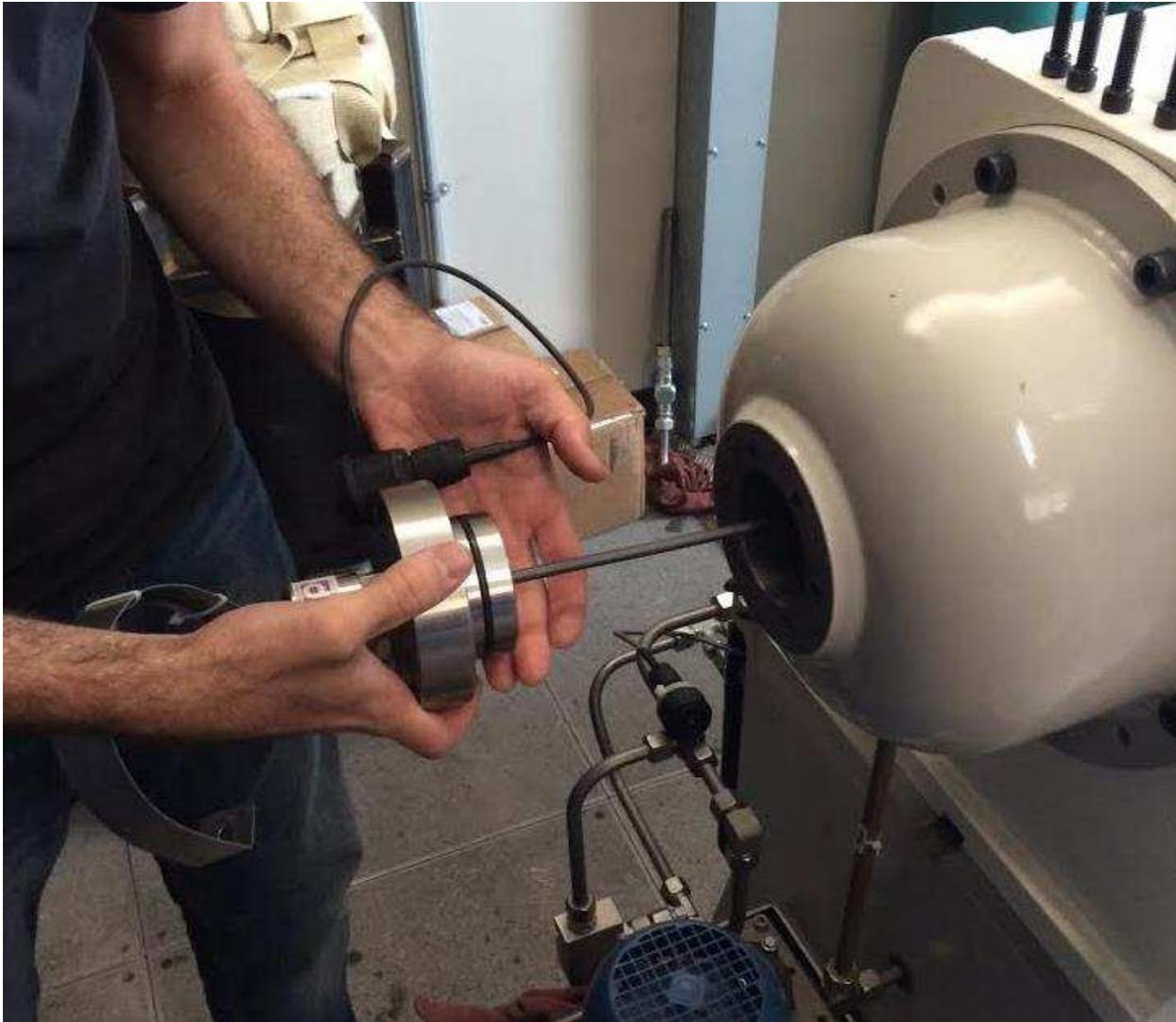
**Figure 8.8 Removing RCM Linear Transducer.**
