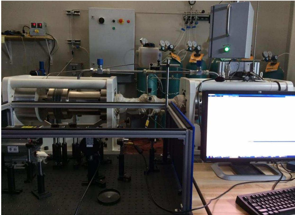
**Figure 2.2 Colorado State University Rapid Compression Machine.**
