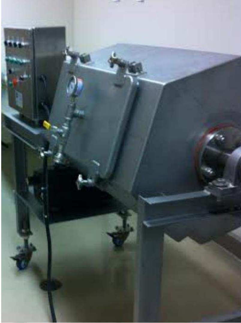
Figure 3.1. Birko-prototype decontamination unit (tumbler) used for both ES1 and ES2.
