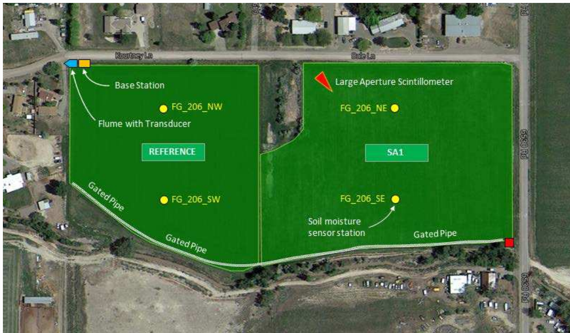
Figure 2 Montrose site; Reference treatment plot on left and Limited treatment plot on right
