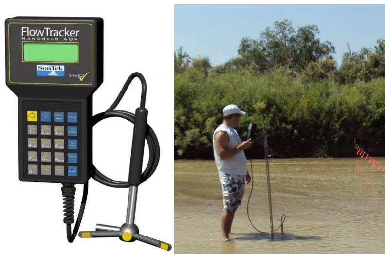
Figure 3-5. (A) A close up of the FlowTracker ( www.sontek.com ) and (B) the FlowTracker and wading rod being used to measure flow.
