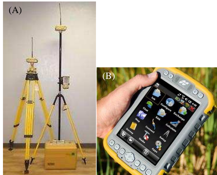
Figure 3-7. Surveying equipment including (A) the base unit (left) and rover (right) and (B) the Tesla data collector ( http://www.gim-international.com/news/id6214-Juniper_to_Manufacture_Topcon_Tesla.html ).
