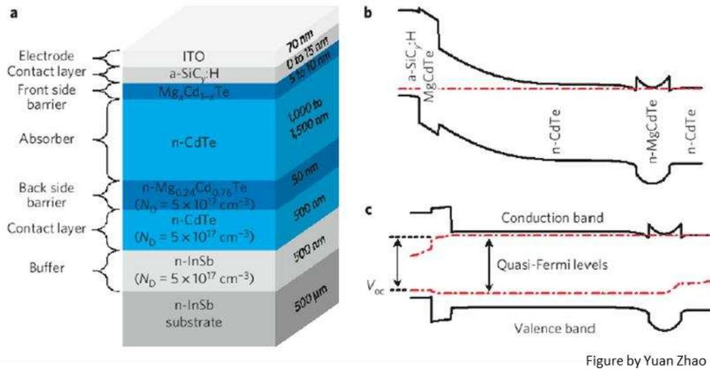
Figure 14: Device design and band diagram, a) layer structure of the CdTe/CMT DHS solar cell. Schematic band diagrams at b) equilibrium c) open circuit (32).
