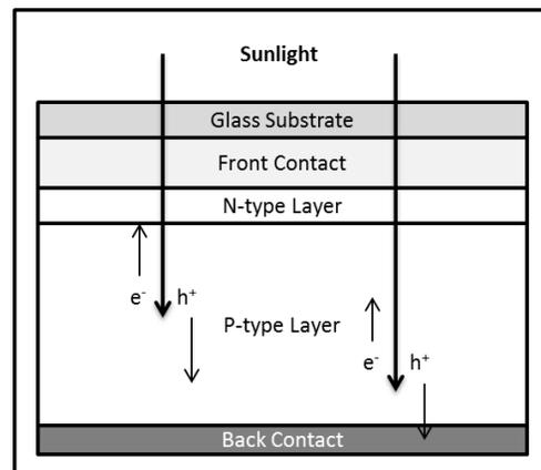
Figure 6: left) The solar spectrum (24) right) A schematic of a simple conventional solar cell, the creation of electron-hole pairs
