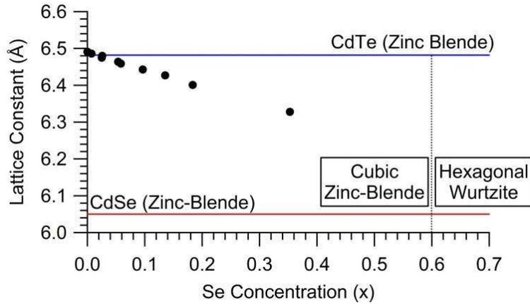
Figure 85: Lattice constant ( $a_0$ ) calculated from XRD as a function of selenium concentration ( $x$ ) with CdTe (Zinc-Blende) and CdSe (Zinc-Blende) referenced (116)
