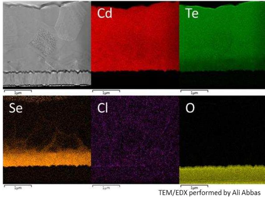
Figure 88 Cross section EDS of a 400 nm 1.45 eV CdSeTe/CdTe device.
