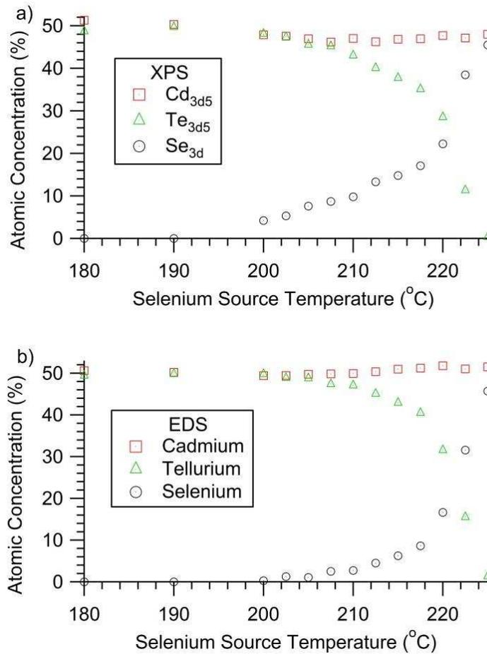
Figure 80: Atomic concentrations of Cd, Te, and Se as measured by a) XPS and b) EDS show increased selenium incorporation at higher temperatures.
