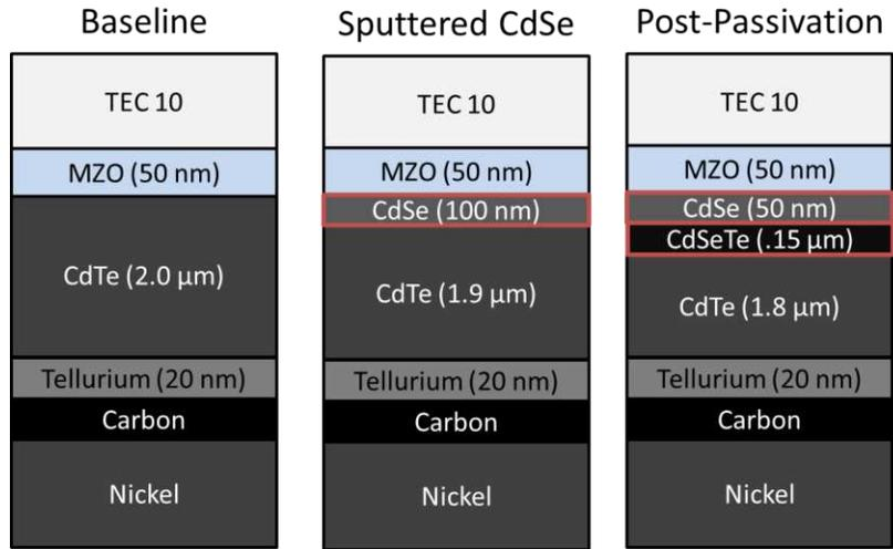
Figure 75: Baseline and Sputtered CdSe Structures
