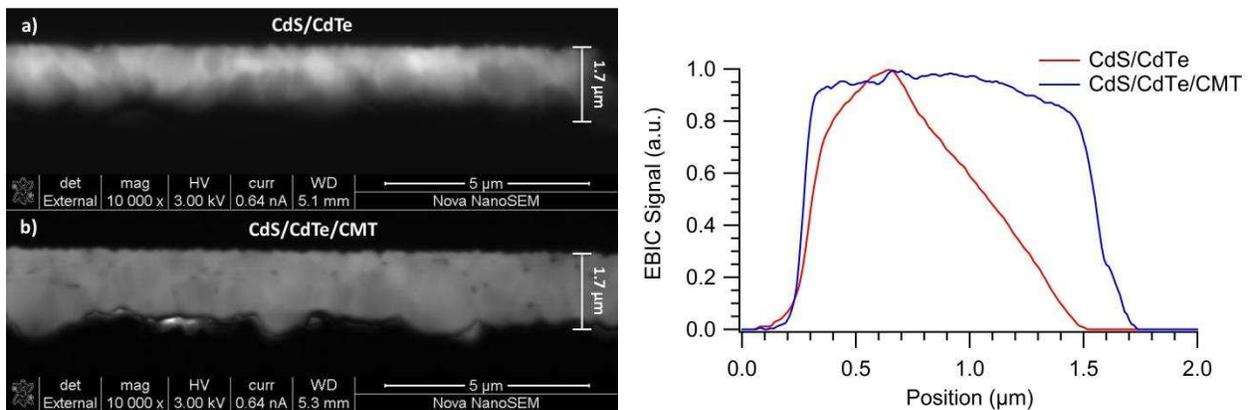
Figure 50: EBIC Maps and line profiles of a) CdS/CdTe (red) and b) CdS/CdTe/CMT (blue)
