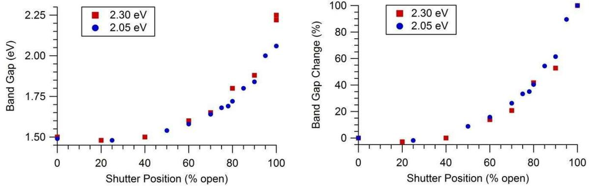
Figure 73: (left) Band gap vs. shutter position, (right) Band gap percent change vs shutter position. (Legend refers to band gap at 100% open shutter position)
