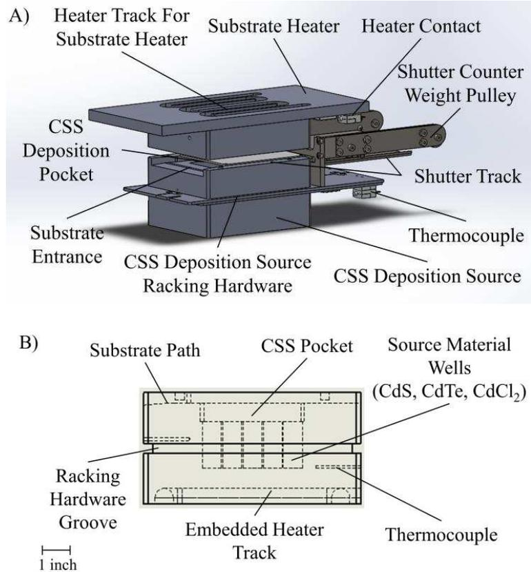
Figure 19 A) CAD of a full CSS source of 1 of 9 typical deposition stations highlighting key components B) A cross-sectional CAD drawing of the bottom deposition source identifying notable features.
