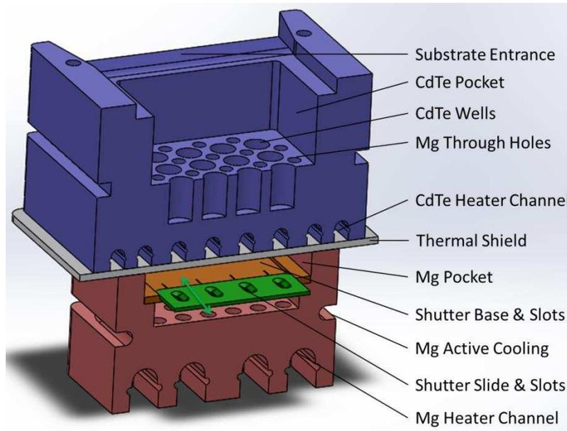
Figure 72: CAD of ARDS Co-Sublimation design with the magnesium shutter design in orange and green.
