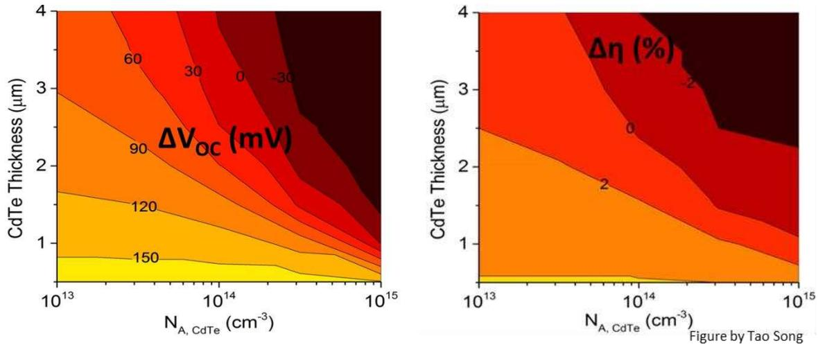
Figure 41: Modeled  $V_{oc}$  vs CdTe doping (82)
