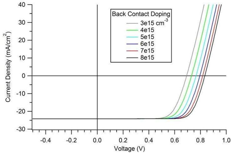
Figure 36: Modeled J-V performance of CdS/CdTe/Telluride cell with various back contact doping (emulating copper migration in ALT)
