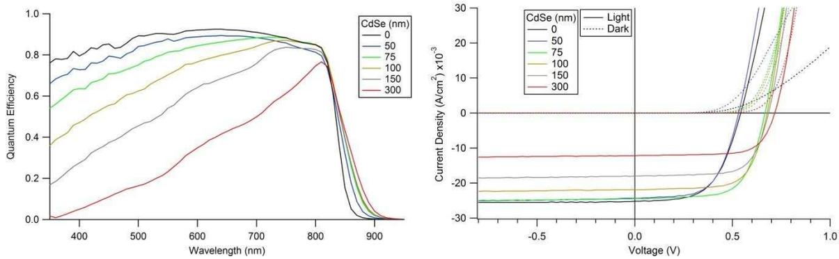
Figure 76: JV and QE of Sputtered CdSe structure with various CdSe thicknesses
