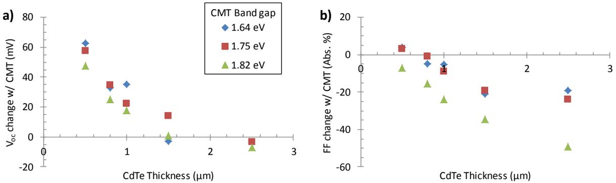
Figure 53: a)  $V_{oc}$  and b) FF change with the addition of the CMT layer at three different CMT band gaps, as a function of CdTe thickness
