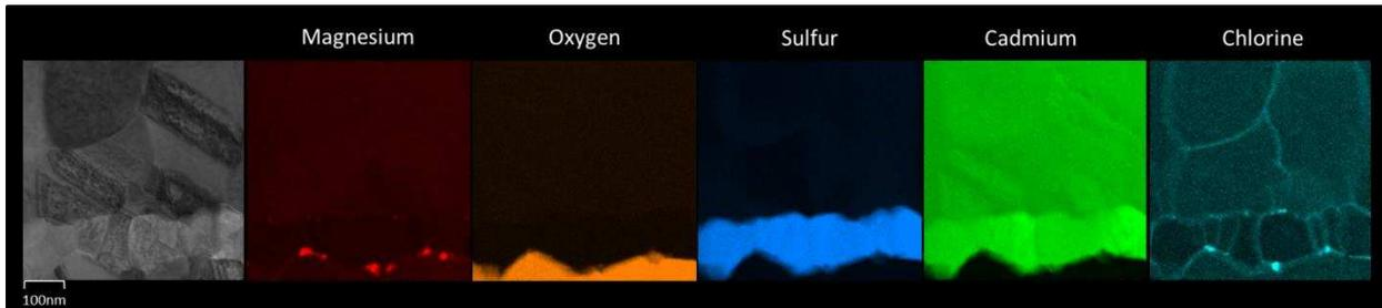
Figure 61: TEM and EDX of the CdS interface of a passivated CdS/CdTe/CMT/CdTe Cap stack.
