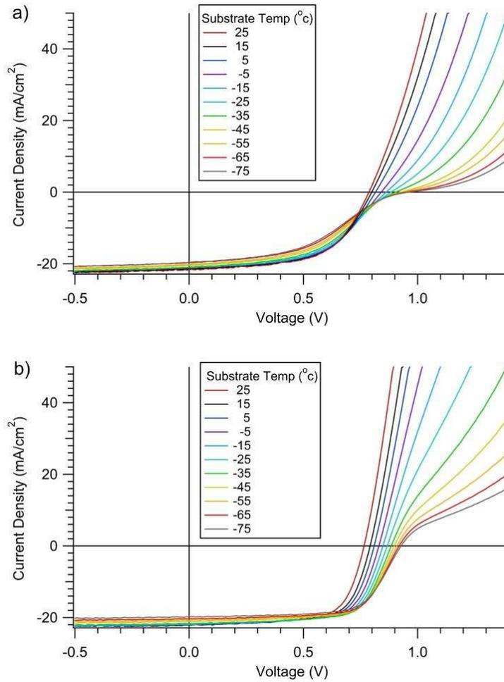
Figure 30: J-V-T of a CdS/CdTe cells with a) carbon paint and b) tellurium.
