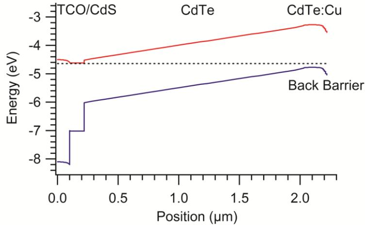
Figure 21: A band diagram of a CdS/CdTe with a low work function back contact and copper doping. Back barrier is an approximation (not to scale).
