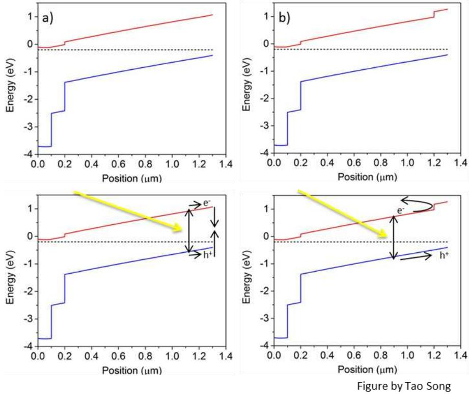
Figure 10: Electron Reflector Concept a) No CBO, b) With a CBO
