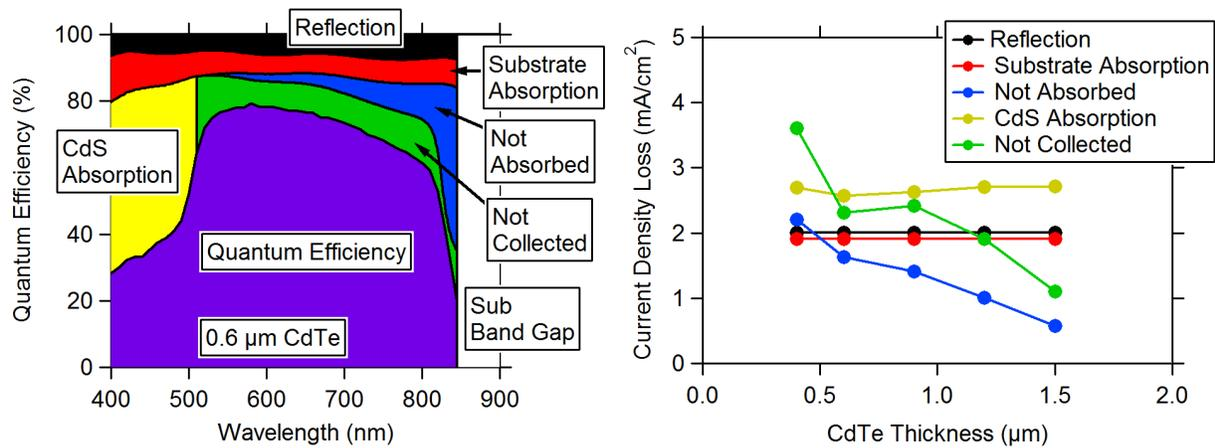
Figure 45: (left) Quantum efficiency of a 0.6  $\mu\text{m}$  CdTe cell (without a CMT layer) illustrating the individual loss mechanisms, (right) Integrated current densities for each category of loss mechanism as a function of CdTe thickness
