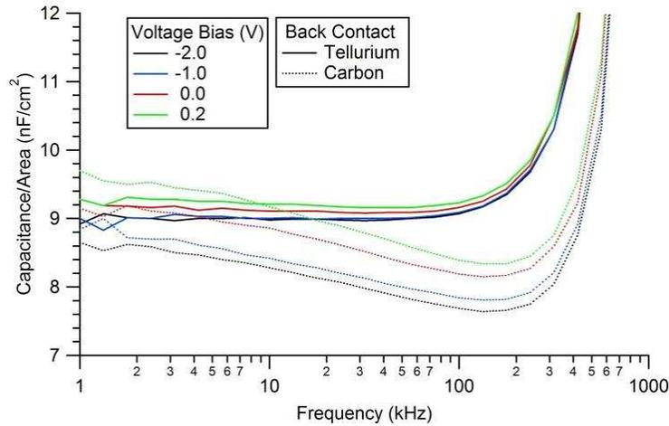
Figure 28: C-F of a CdS/CdTe baseline cells with tellurium vs carbon back contacts, showing a significant improvement in dispersion with the tellurium back contact.
