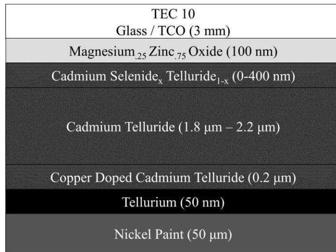
Figure 86: CdSeTe/CdTe structure to assess the CdSeTe ability to collect photons below 820 nm.
