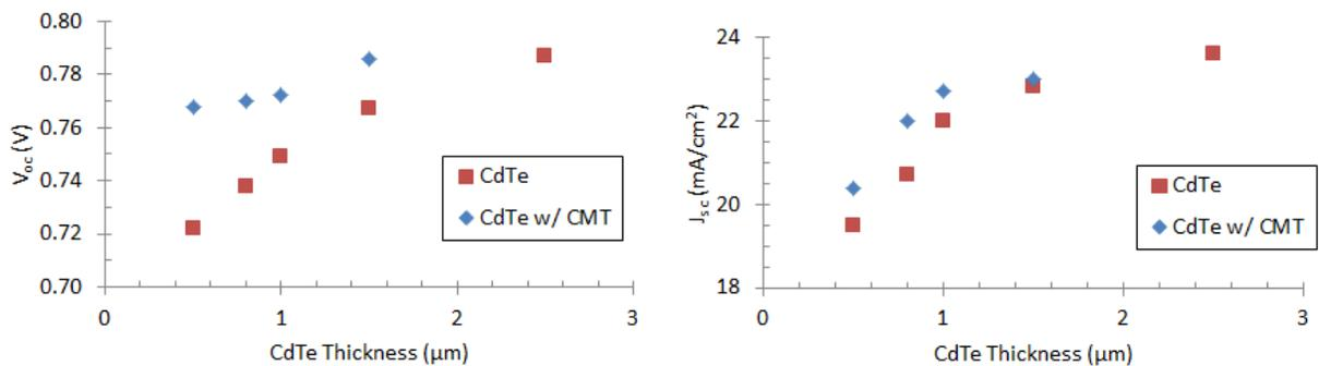
Figure 47:  $V_{oc}$  and  $J_{sc}$  of CdS/CdTe cells at various CdTe thicknesses; with (Blue Diamonds) and without (Red Squares) a 1.75 eV CMT film
