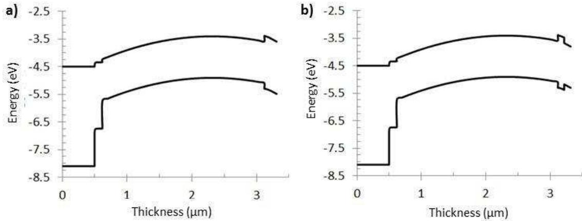
Figure 54: Band Diagram of a) TCO/CdS/CdTe/CMT/Carbon and b): TCO/CdS/CdTe/CMT/CdTe Cap/Carbon
