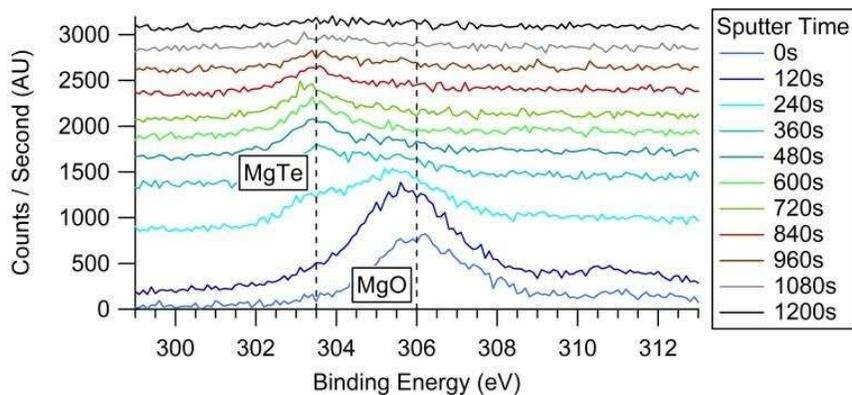
Figure 57: XPS of the Magnesium KLL peak, (Sputtered from bottom to top)
