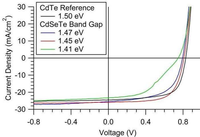
Figure 90: JV of 1.47, 1.45, and 1.41 eV CdSeTe/CdTe cells at 200 nm CdSeTe thicknesses.
