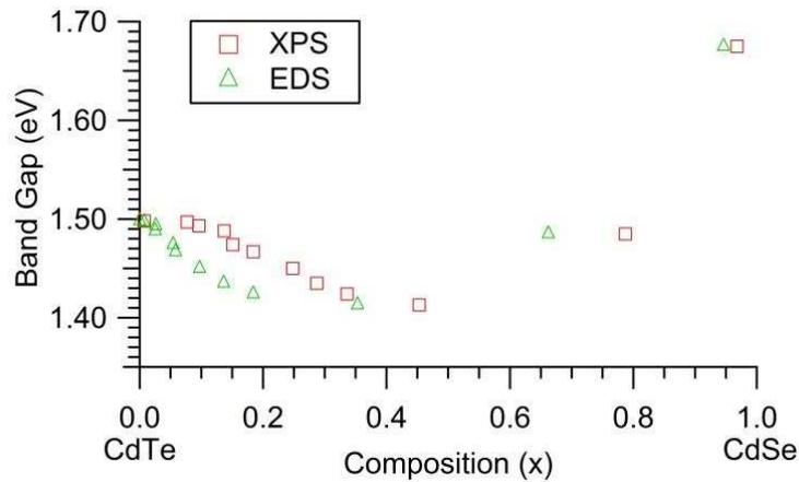
Figure 81: CdSeTe band gap as a function of selenium concentration as measured by XPS and EDS.
