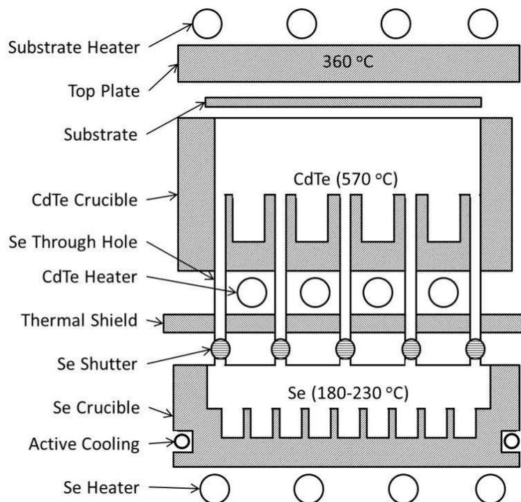
Figure 78: Co-sublimation hardware for alloying CdTe and selenium (Gen IV). The selenium vapor pressure is directed into the CdTe pocket to allow sublimation of the alloy.
