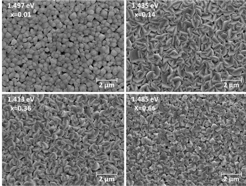
Figure 82: SEM images at  $x = 0.01, 0.14, 0.36,$  and  $0.66$ . A clear change in morphology is seen as the selenium concentration is increased. Se concentration  $x$  is estimated from EDS.
