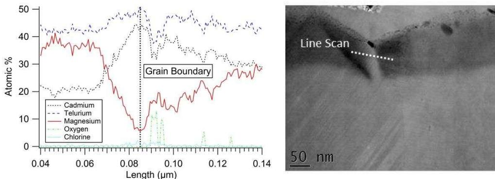
Figure 60: Line scan of a CdS/CdTe/CMT/CdTe Cap stack grain boundary passivated with  $\text{CdCl}_2$
