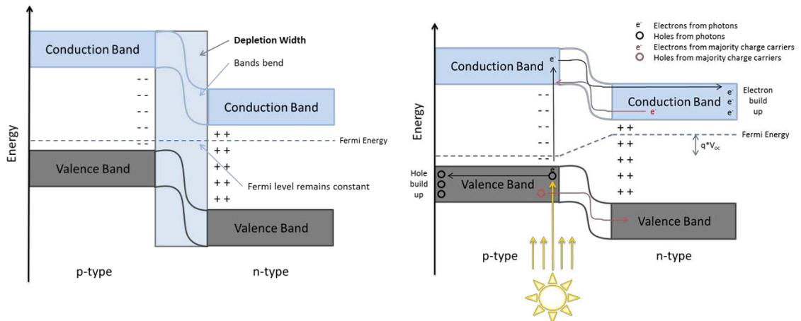
Figure 8: a) The p–n junction b) p-n junction under photon bias.
