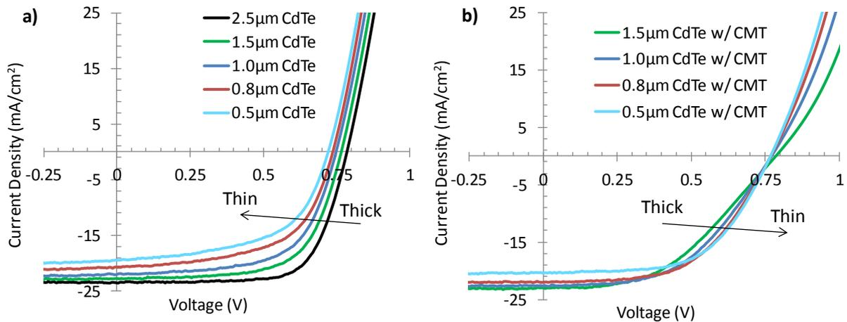
Figure 44: J-V Curves of a) CdS/CdTe and b) CdS/CdTe/CMT cells with various CdTe thicknesses
