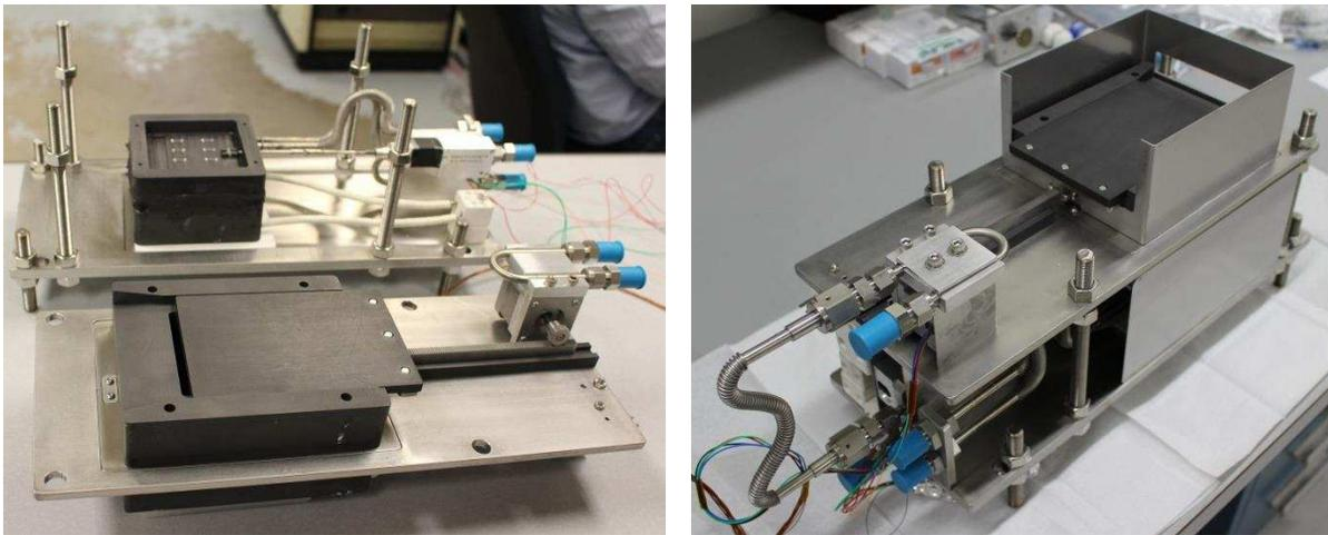
Figure 71: Images of ARDS Co-Sub design, (left) Magnesium and CdTe sources shown separately (right) the completed co-sub source.
