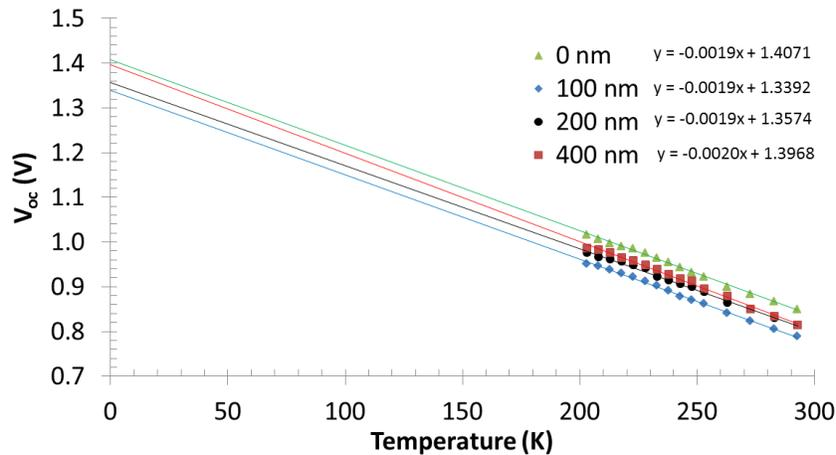
Figure 93: Temperature dependent JV for 1.45 eV CdSeTe cells with varying CdSeTe thickness.
