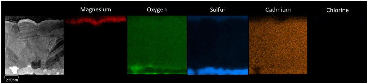
Figure 55: Cross Section TEM and EDX of CdS/CdTe/CMT stack without passivation
