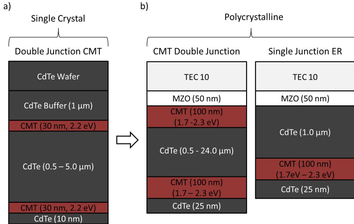
Figure 64: Double hetero-structure CMT/CdTe/CMT a) Single Crystal b) Polycrystalline
