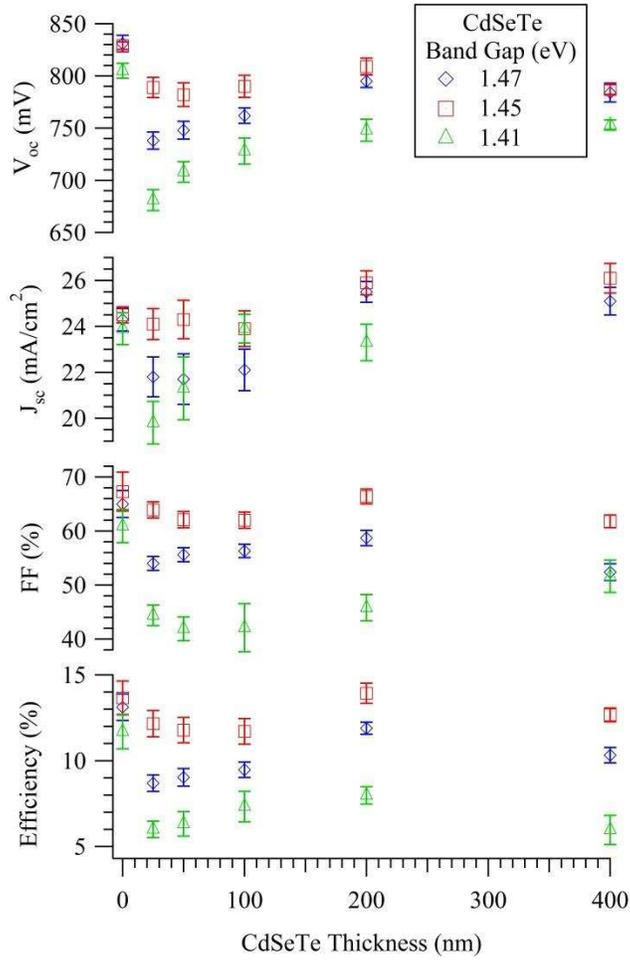
Figure 89: JV performance parameters of MZO/CdSeTe/CdTe devices with the CdSeTe layer at 1.47, 1.45, and 1.41 eV. The CdSeTe thickness is swept from 0 – 400nm. Average device values are used with a plus/minus one standard deviation error bar. J<sub>sc</sub> at 1.41 eV and 400 nm is 15.4 mA/cm<sup>2</sup>.
