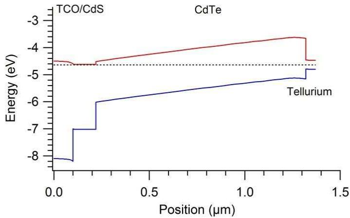
Figure 33: Band diagram of a CdS/CdTe cells with a tellurium back contact, the barrier is formed in the opposite direction of the carbon back contact cell.
