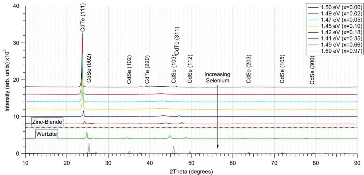
Figure 83: Glancing Angle (1.5°) XRD at varying selenium concentrations, showing the shift from a cubic to hexagonal structure.
