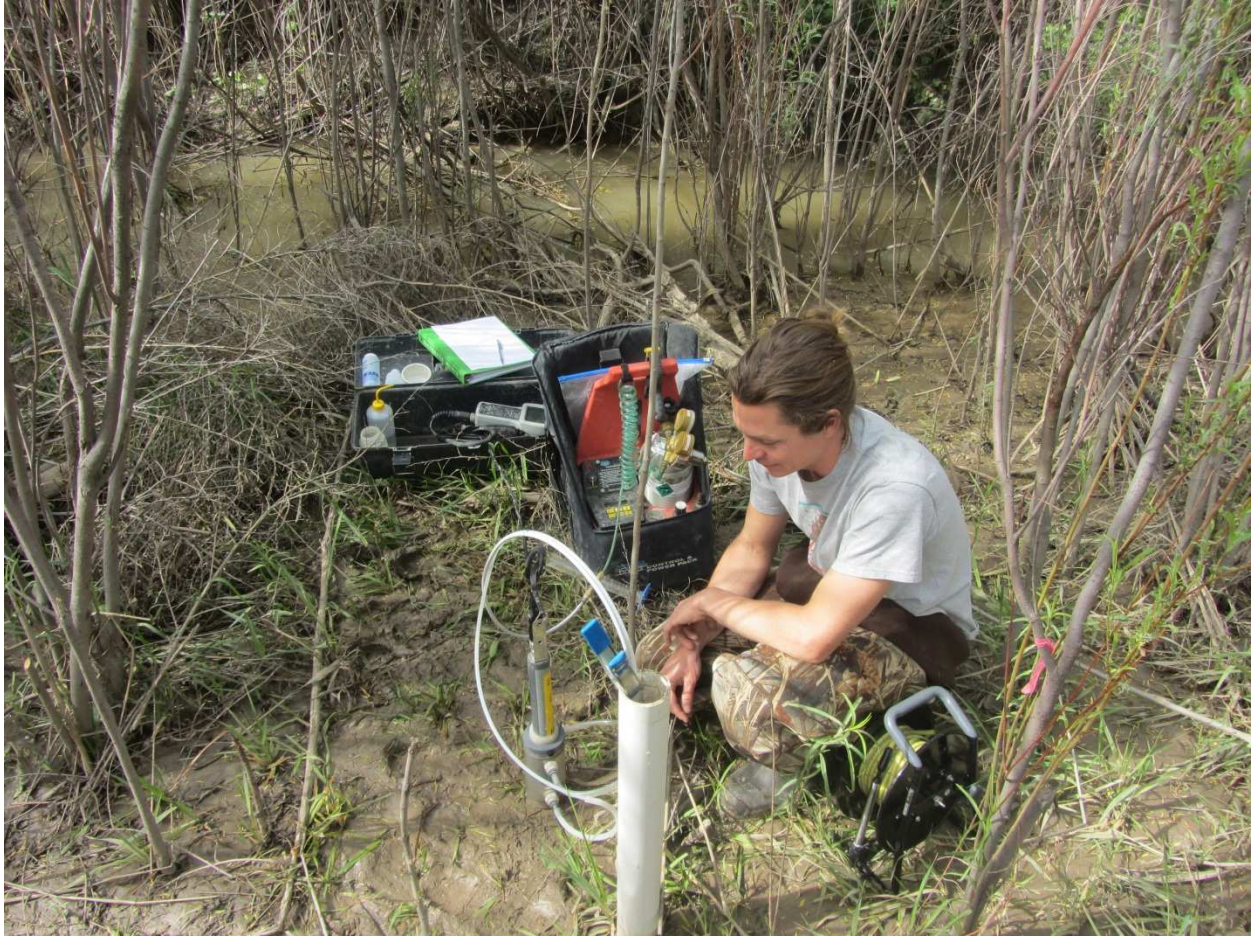
Figure 9. Waiting for in-situ water quality parameters to stabilize using the YSI sonde and flow-through cell before collecting a groundwater sample at monitoring well ARKB2.
