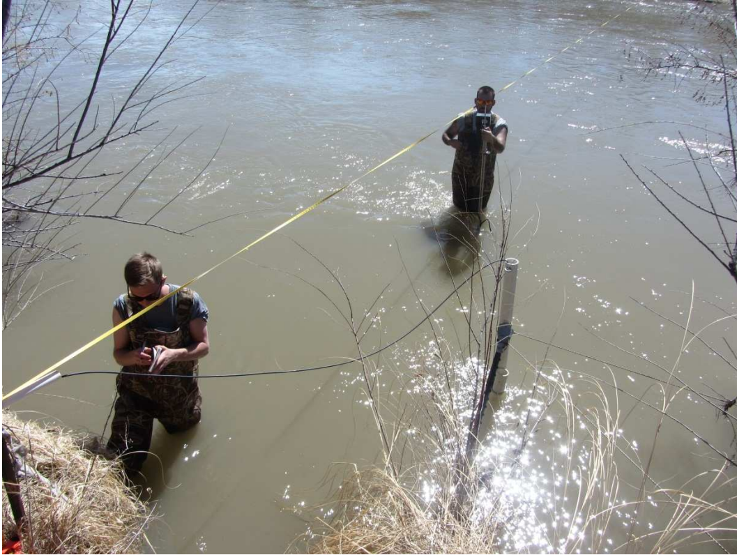
Figure 8. Streamflow gauged along the river cross-section of transect ARKD using an ADV. Field notes were also recorded.
