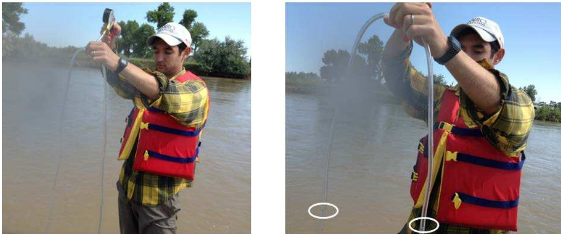
Figure 11. Negative pressure was applied equally to PushPoints™ using the hand pump and T-connector.
