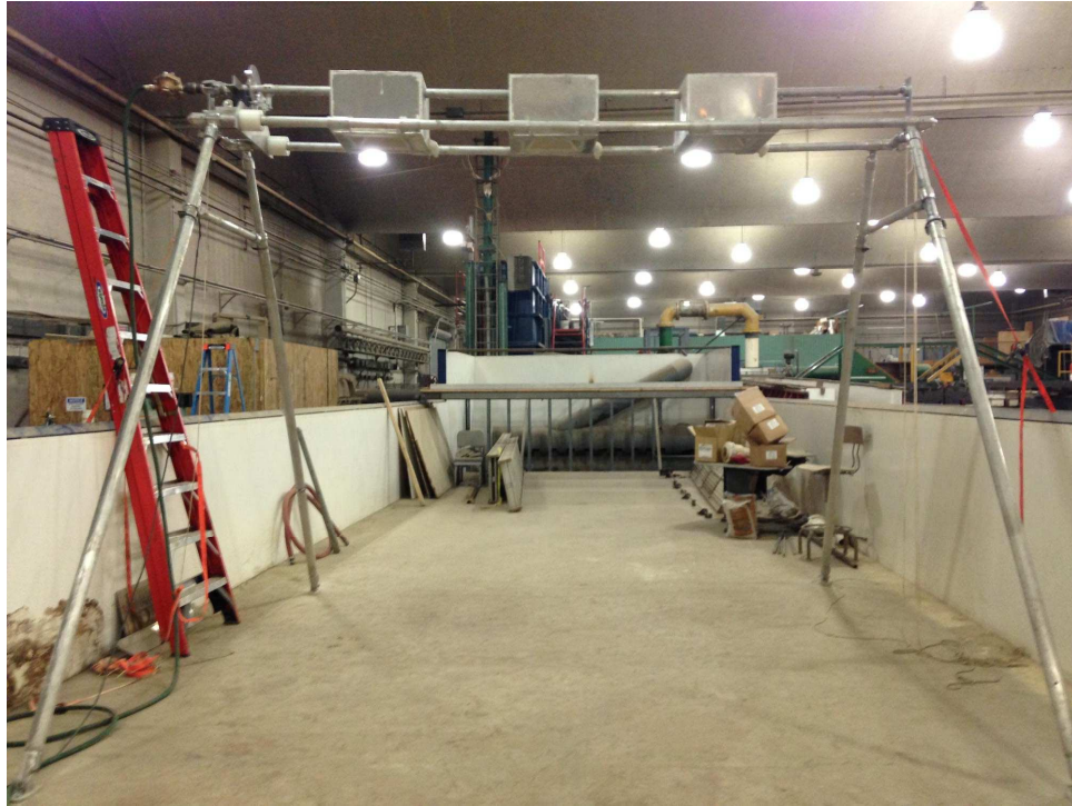
Figure 2.2 Norton Ladder Type Rainfall Simulato
