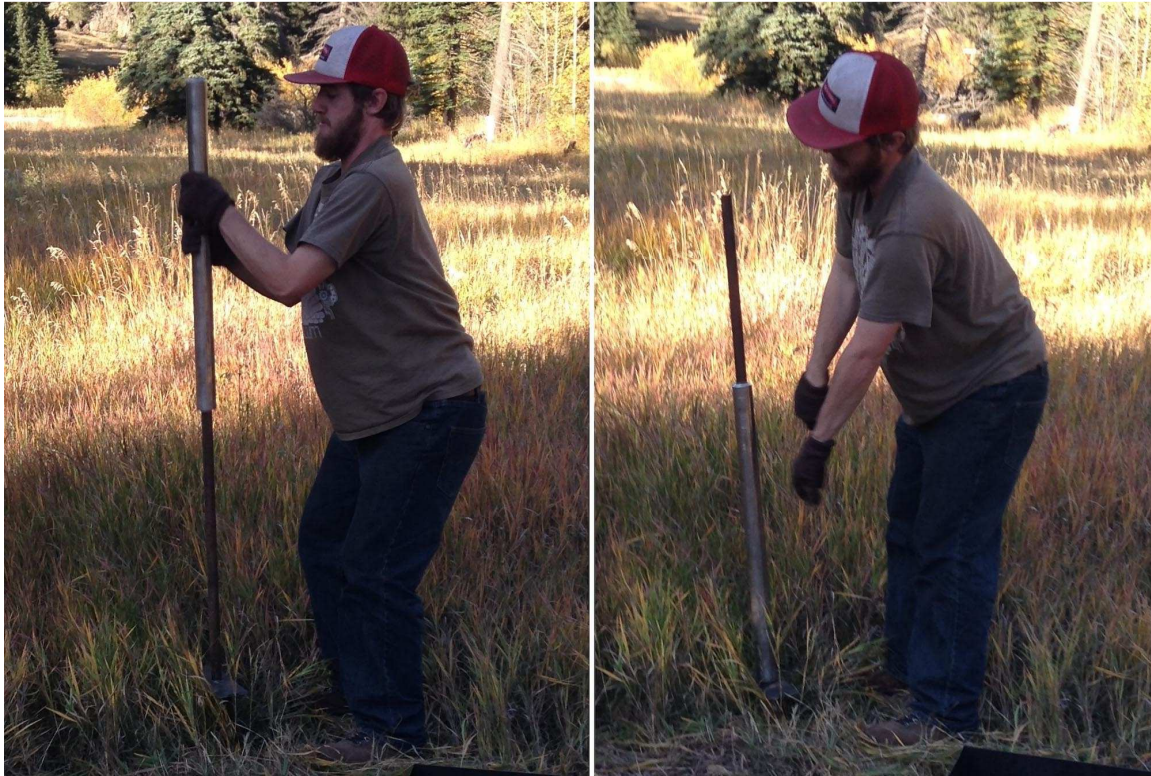
Figure 2.1 Use of slidehammer to indent dimensions of the soil plot
