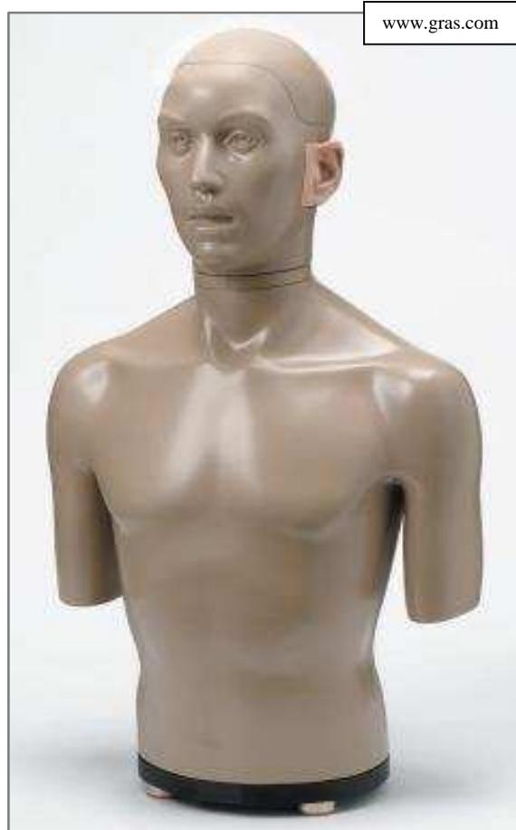
**Figure 5.2: Knowles Electronic Manikin for Acoustical Research (KEMAR) Type 45 BA**
