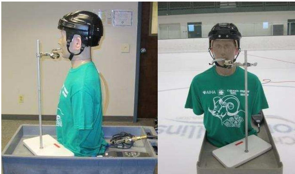
**Figure 5.5: KEMAR sampling assembly (left) a. side view of KEMAR Type 45 BA assembly fitted with a Bauer hockey helmet, Fox 40<sup>®</sup> Super Force<sup>®</sup> finger grip pea whistle apparatus, and the Larson Davis SLM/OBA; (right) b. front view of KEMAR assembly located on the ice at a northern Colorado ice rink**
