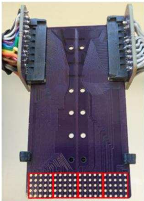
Figure 16: The electrode array on an assembled mouthpiece shown divided into four 5x5 sub-arrays.
