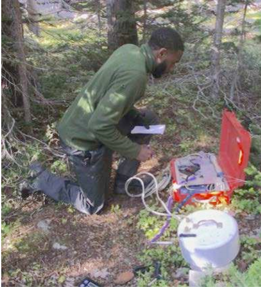
Figure 4. The author using a Li-Cor LI82 to measure soil respiration in Loch Vale watershed, Rocky Mountain National Park.
