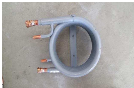
Figure 26: (A) Original Fan-Cooled Condenser (B) Water-Cooled Condenser
