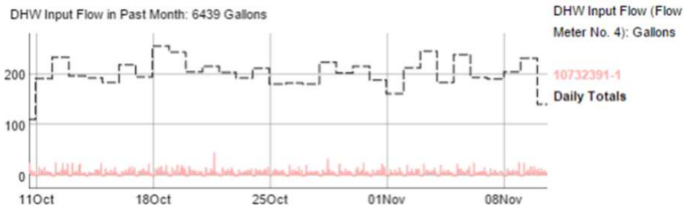
Figure 16: Starbucks Store #14944 Domestic Hot Water Use
