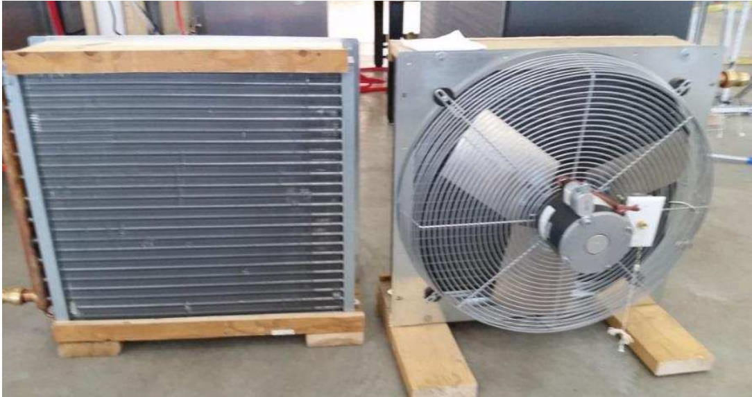
Figure 36: Heat Rejection System
