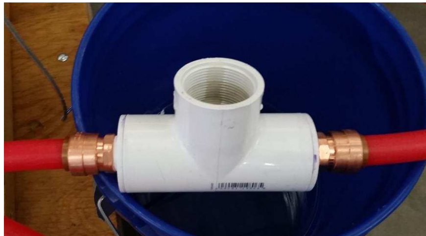
Figure 12: Temperature Logger Insertion Point
