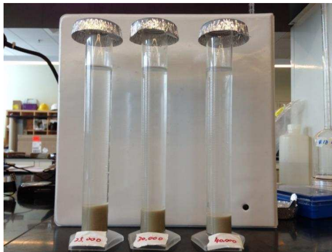
Figure G-2. Clay swelling test set up with TDS from 25,000 to 40,000 mg/L
