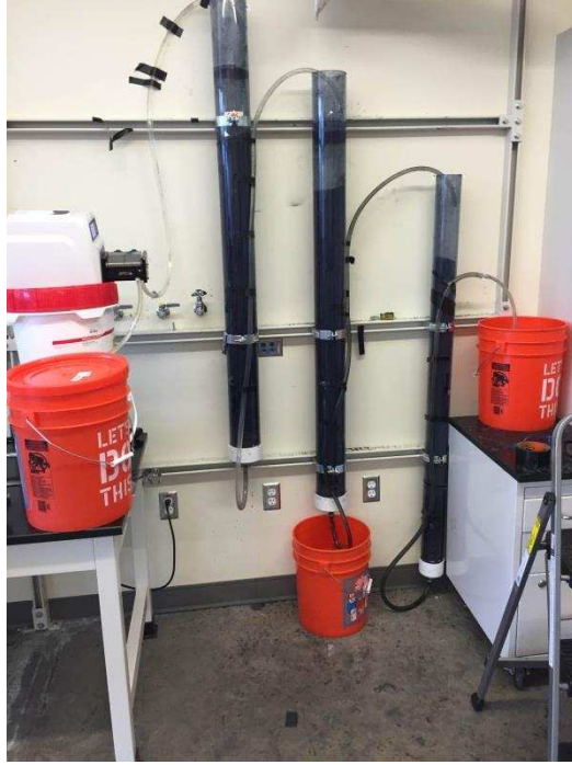
Figure 3-6: Granular Activated Carbon Columns in Series at CSU Laboratory
