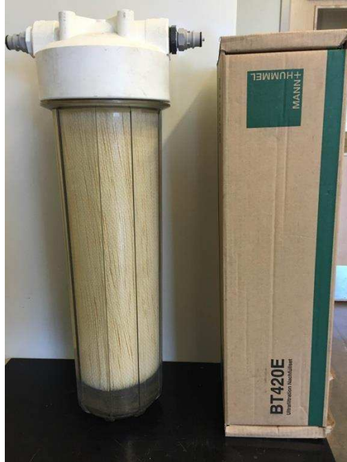
Figure 3-5: Hollow Fiber Ultrafiltration Unit
