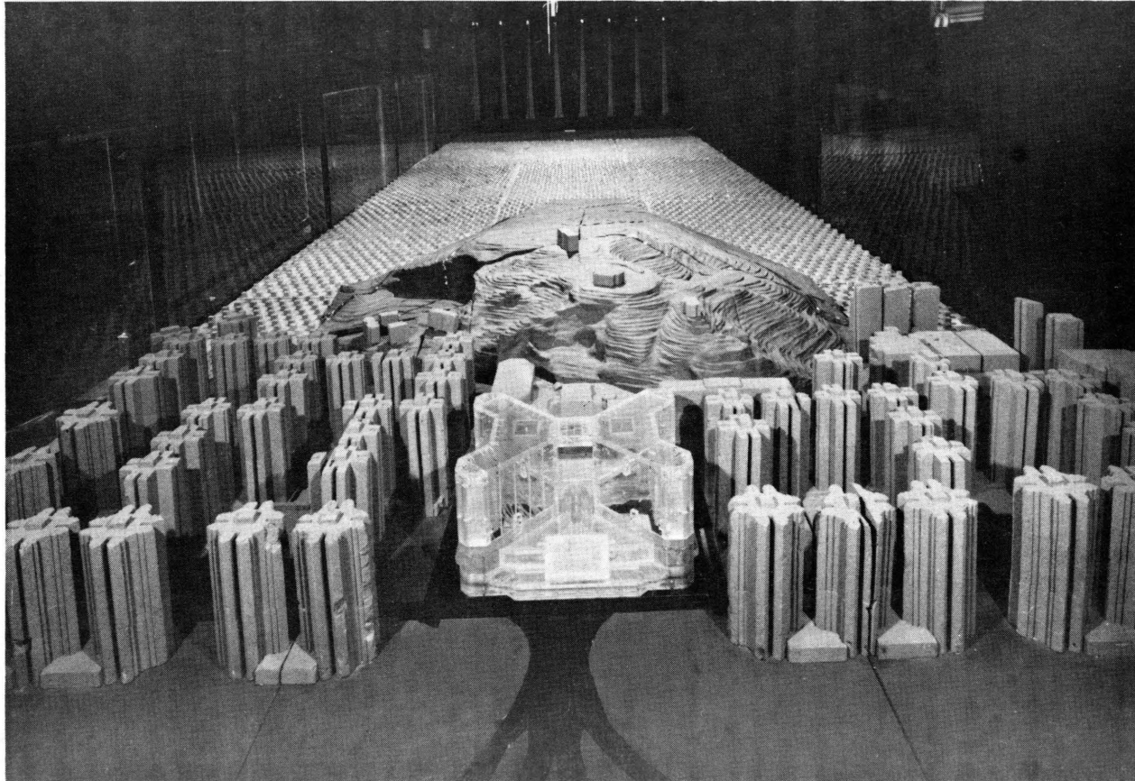
Figure 5. Model Installed in the Wind Tunnel
