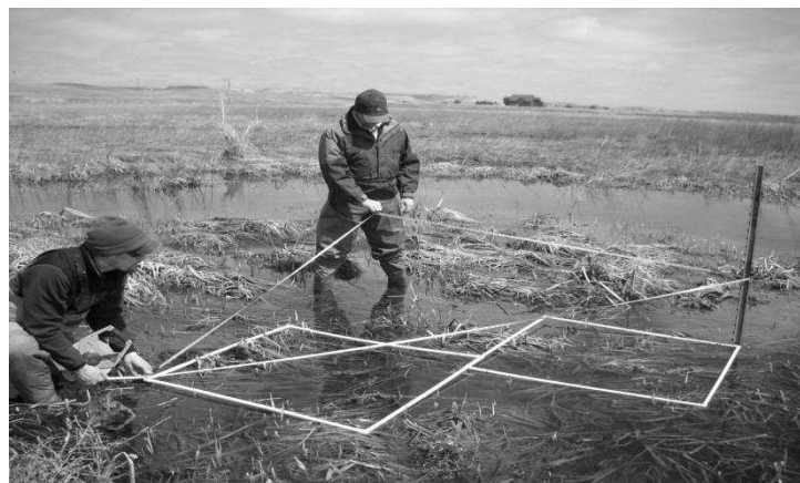
Figure 1. Plot layout- Plots were marked with two t-posts and were laid out by forming a right isosceles triangle with a tape measure. The right isosceles triangle had a hypotenuse 2.82 meters ( \sqrt{2} * A =
