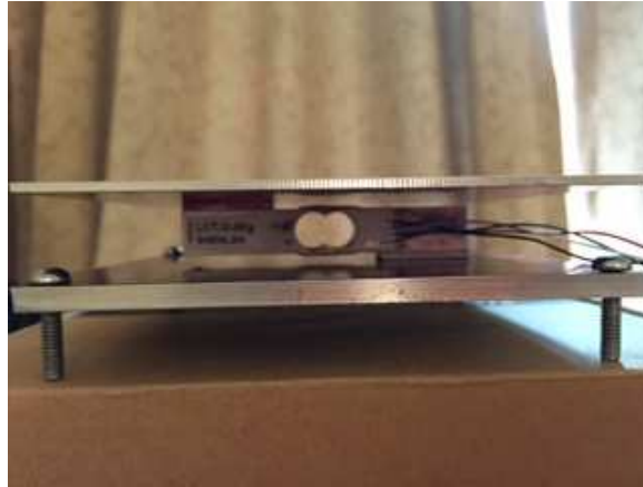
Figure-22 Metal platform and 5kg load cell
