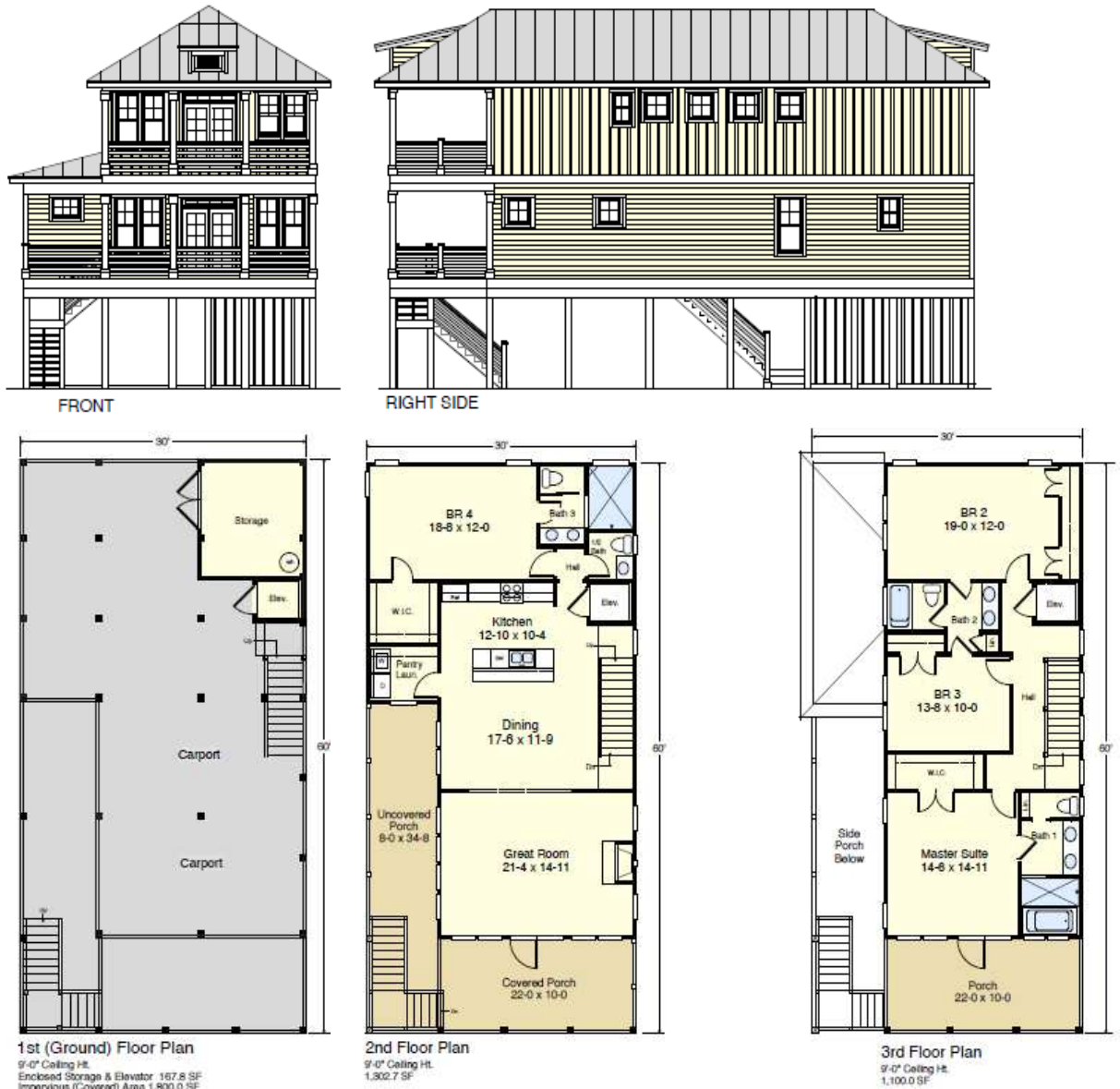
Figure 7-18. Example of two –story elevated building in Carolina Island
