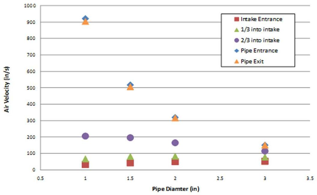
**Figure 2.6:** Relative airspeed velocities at various depths of the port compared to pipe diameter.
