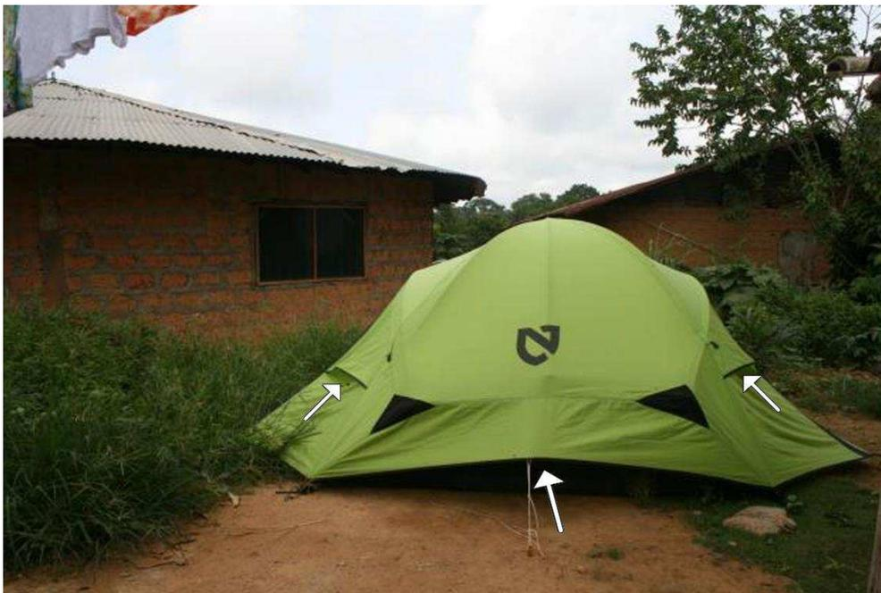
**Figure 3.1:** Infoscitex Tent in “location 1” of Bolahun, Liberia. Three openings for mosquito entry on this side are marked.
