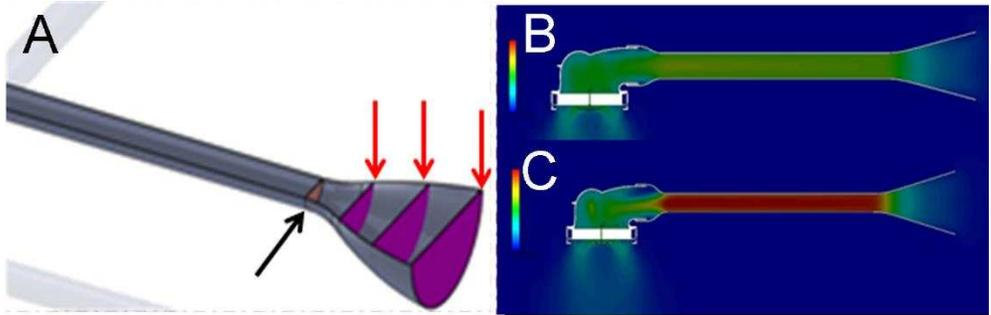
**Figure 2.5:** (A): Layout of the reference planes (red arrows) in CFD simulation models. Black arrow indicates final tube (pipe) diameter. (B and C): Cross section cut plot of air velocity in of 2” diameter x 20” Long tube and a 1.5” x 20” Long Tube, respectively.
