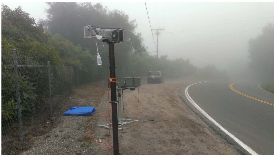
Figure A3-1. Example sampling setup demonstrating deployment of CASCC2 (left) and ss-CASCC (right) as well as location with respect to road and campaign vehicle.
