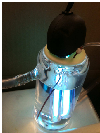
Figure 1-8. Photoreaction vessel used in the study of aqueous atmospheric oxidation processes of organics (e.g., in Boris et al., 2014). Recirculating water jacket inlet is pictured on the left of the vessel; UV-C light source is u-shaped bulb submerged into solution; outlet for online MS analysis is brown tubing placed into reaction solution.
