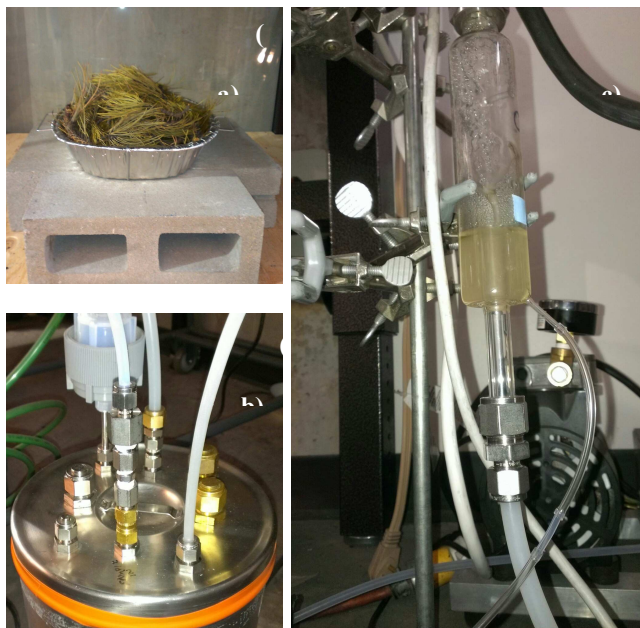
Figure A6-1. Photos of setup for simulated burns and collection of smoke: (a) burn platform with fuel in hood; (b) mixing chamber with connections to filter pack, CO, zero air inlet, and waste air outlet; (c) mist chamber with water containing emissions from burns (air flows upward through apparatus, causing spray of water to form and drip down walls).
