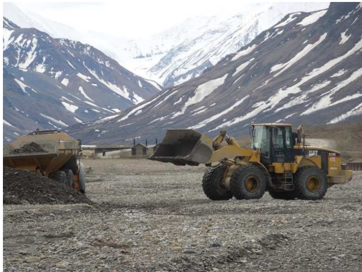
Figure 6: An excavator dumps recently excavated sediment into a rock truck that will transport the material to the adjacent Road Camp along the Toklat River. View is south and upstream.
