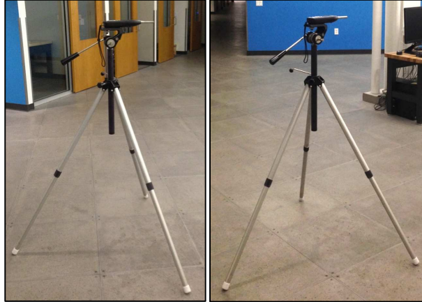
Figure 4.2: SLM mounted on tripod. SLM mounted perpendicular to floor at a height of 54 inches for all measurements.
