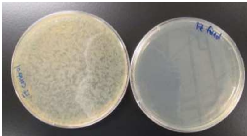
Figure 5.1: Complete sterilization of F. tularensis following a 5 minute exposure to 4% PFA can be observed on the right plate and a lawn from the untreated vial can be seen on the left plate.
