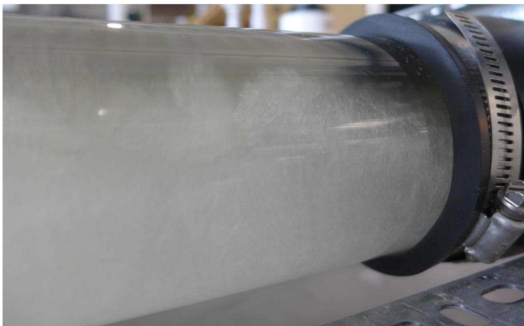
Figure 35. Enhanced view of \text{Na}_2\text{CO}_3 \cdot 10\text{H}_2\text{O} crystal growth in pipe.
