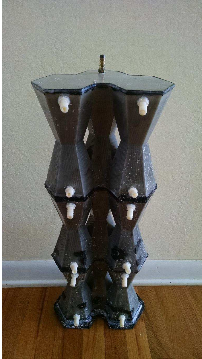
Figure 29. Crescent design with TFAD post processing and all hose barbs (printed and metal) installed.
