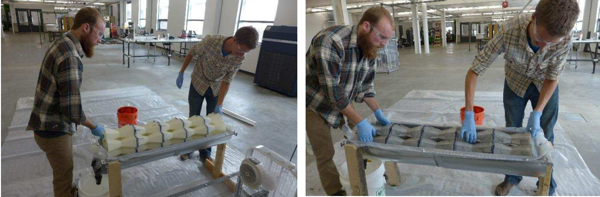
Figure 28. Demonstration of TFAD technique of the full hexagon design and the size, shape, and number of components of the unit. The assembly of printed components prior to TFAD was rejected after this test as the amount of ABS solution required is far greater than TFAD of the individual components prior to assembly.
