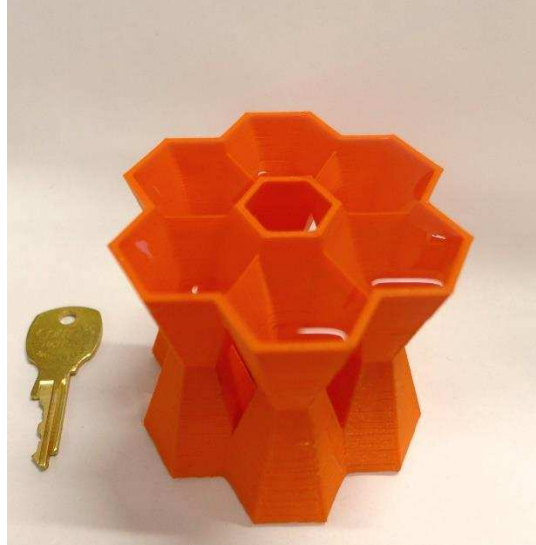
Figure 24. Waterproof hexagon pattern with prism spacing test coupon (Full hexagon design.)
