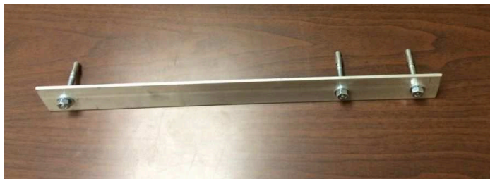
Figure 2. Scratching Piece for Scratch Gauge ( Part 2 )
