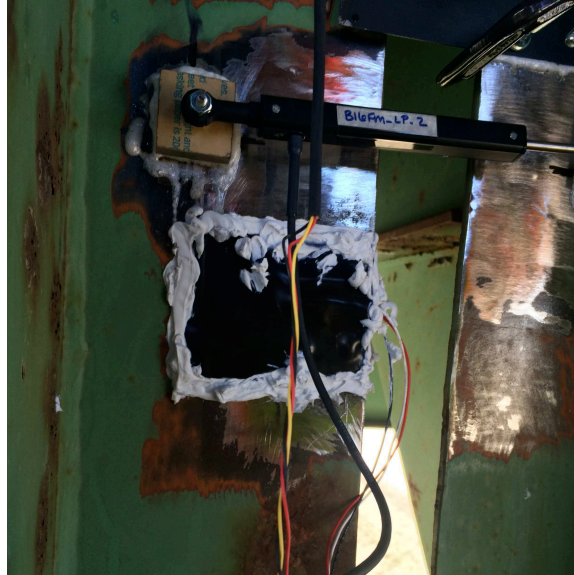
Figure 3-21. Covered Strain Gauge using Butyl Rubber Vinyl Barrier E
