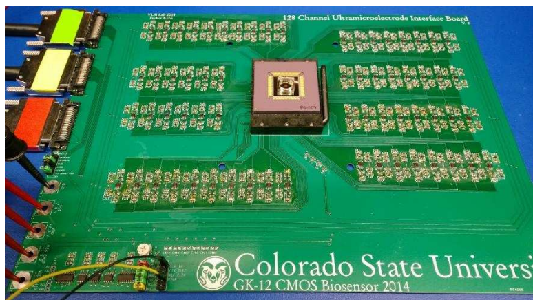
Figure 5.9: Circuit board with the electrode array chip in the middle and other supporting circuits around it.
