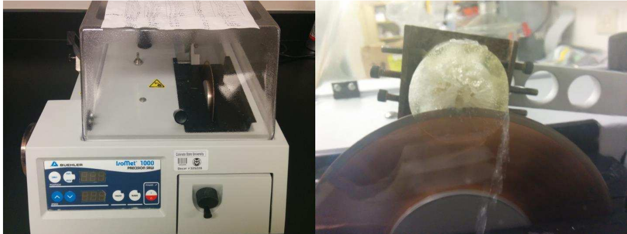
Figure 13: Left shows the Buehler IsoMet 1000 that was used to finely section the bones into 300 micron slices. Right shows the IsoMet 1000 cutting a sample.
