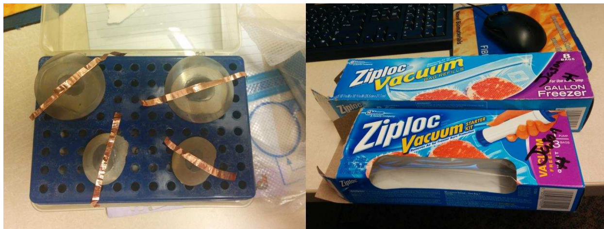
Figure 15: Left shows the modified tips box and the general use of copper tape. Note: the copper tape may not be in the right orientation. It is extremely sticky and sometimes pulls off in the removal of the sample from the grounding plate. Since these samples were done the copper tape was put back on to hold them in the box, orientation was not taken into account. Right shows the vacuum system to transport the samples to the SEM, on the day of scanning.
