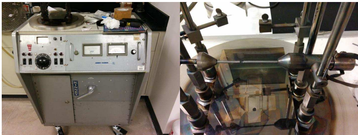
Figure 16: Shows the carbon depositor. Left is a picture of the entire instrument, minus the glass bell. Right, is a close up of the platform and the carbon rods, being pressed together.
